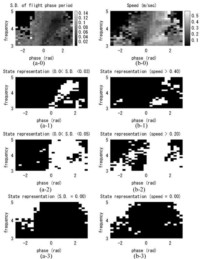
Fig. 7. Behavior landscape obtained by a ground contact detector (a-0), and the visual velocity detector (b-0). This landscape is then segmented by threshold in (a-1-3) and (b-1-3).
