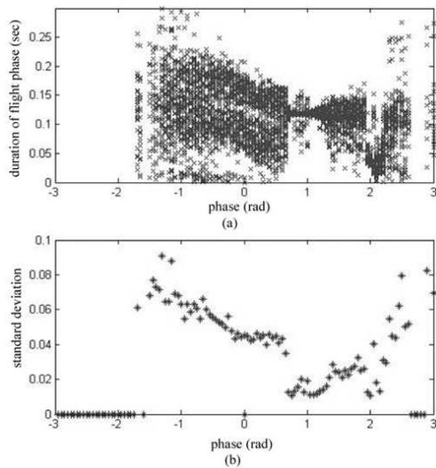
Fig. 6. Body dynamics during the locomotion experiment measured by a contact detector. (a) distribution of the flight phase durations against the phase parameter, and (b) its standard deviation (SD).  $SD = 0$  indicates that the running behavior is not possible with the corresponding control parameter.
