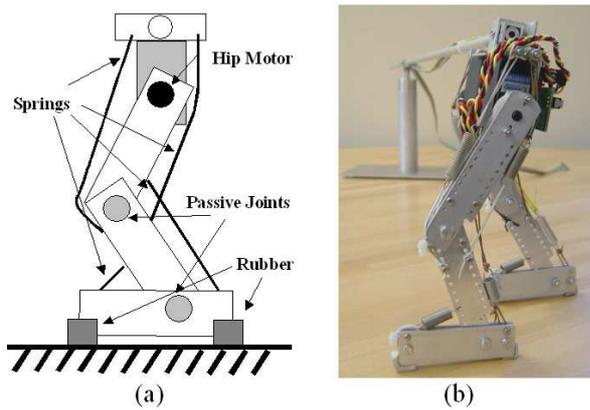
Fig. 1. (a) Schematics of the robot design, (b) photograph of the robot with the supporting rotational bar.
