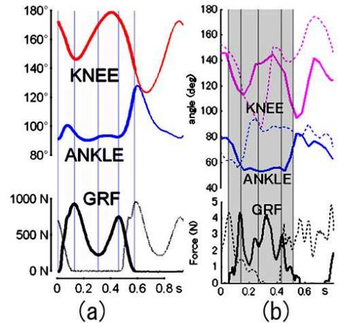
Fig. 3. Angular trajectories of the knee and the ankle joints and the ground reaction force of human locomotion(a), and of the robot(b).
