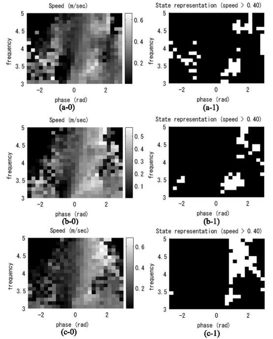
Fig. 9. The different dynamics observed by the speed detector with respect to the different ground friction of (a) 0.5, (b) 0.65 and (c) 0.8. The landscape is then segmented by threshold in (a,b,c-1).
