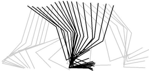
Fig. 2. Leg trajectory of the biped robot during one step. Black and gray lines depict right and left legs, respectively.
