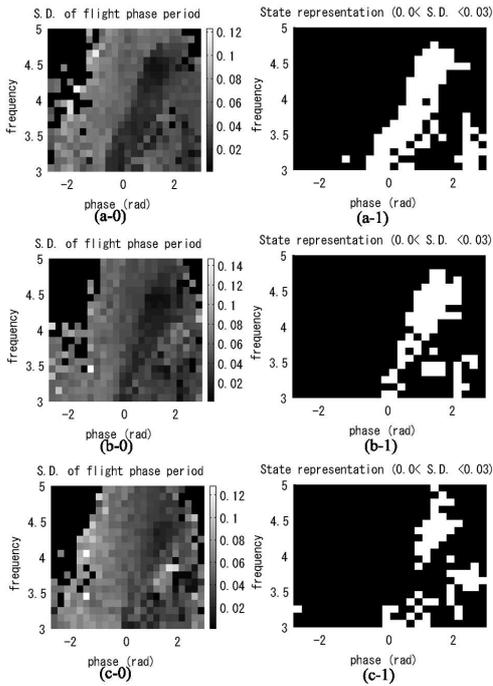
Fig. 8. The different dynamics observed by the contact detector with respect to the different ground friction of (a) 0.5, (b) 0.65 and (c) 0.8. The landscape is then segmented by threshold in (a,b,c-1).
