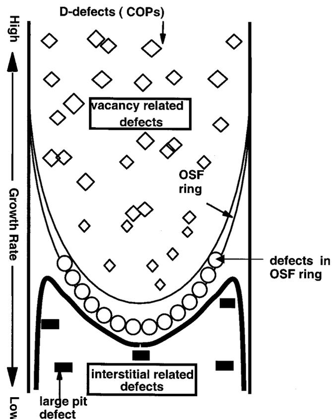
Figure 1. Grown-in defects in a silicon crystal, grown with a varying pulling rate.
