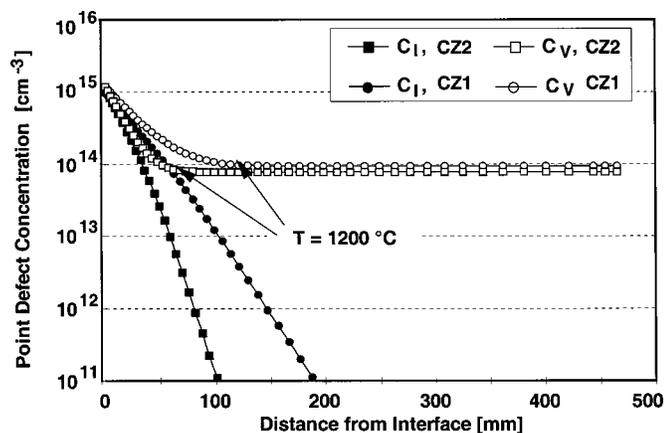
**Figure 3.** Vacancy ( $C_V$ ) and self-interstitial ( $C_I$ ) concentrations in growing CZ silicon crystals (CZ1 and CZ2) as a function of distance from the solidification interface.
