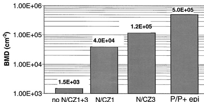
**Figure 10.** BMD densities after process simulation of wafers from non-nitrogen and nitrogen doped CZ1 and CZ3 crystals and of p/p<sup>+</sup> wafers.
