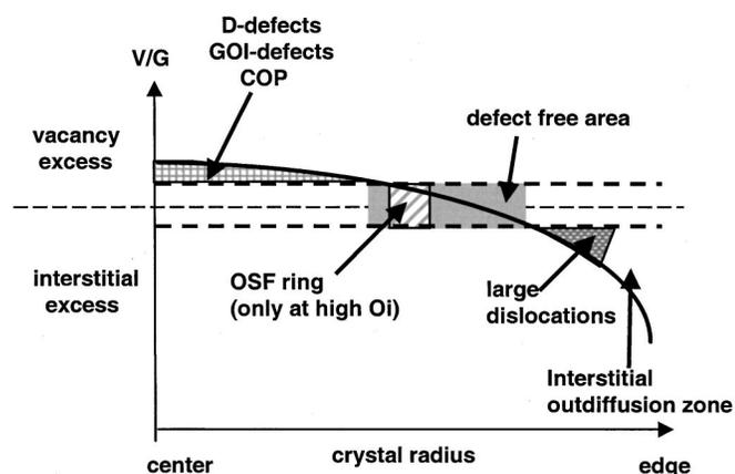
**Figure 2.** Radial variation of  $V/G$  in CZ silicon crystals grown with a transition from vacancy-rich to interstitial-rich from center to rim.
