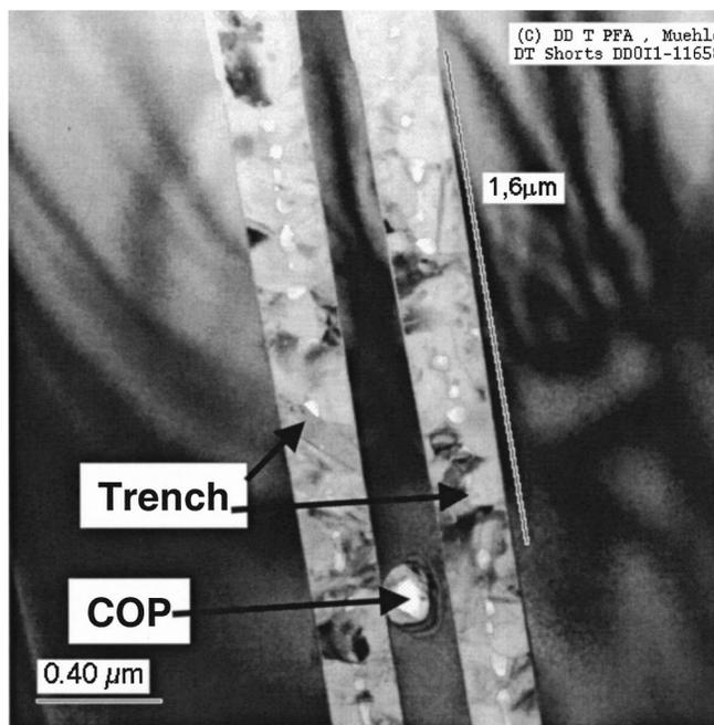
**Figure 6.** Scanning electron microscope (SEM) image of a COP short fail between adjacent deep trenches of an actual fabricated DRAM product, clearly showing the storage dielectric and poly electrode fill and the empty space in the COP center. Trenches are located above and below the photograph level.
