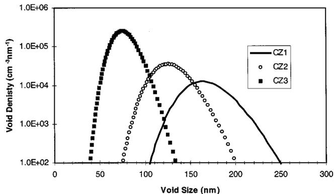
**Figure 4.** COP distributions in slowly (CZ1), medium (CZ2), and fast (CZ3) cooled 200 mm crystals.
