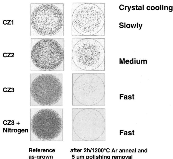
**Figure 9.** COPs on as-grown and annealed polished wafers from CZ1, CZ2, CZ3, and nitrogen-doped CZ3 crystals.
