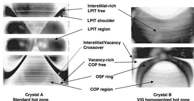
**Figure 8.** Defect distributions (after heat-treatment and etching) in crystals A and B grown with pull rate ramps in a standard and in a  $G$  homogenized hot zone, respectively.
