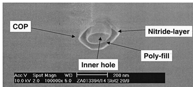
**Figure 7.** Transmission electron microscopy (TEM) image of a COP short between adjacent deep trenches of an actual fabricated DRAM product. The cut with the right trench is located outside the TEM sample cross section shown.
