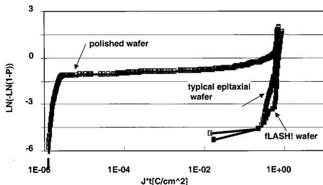
**Figure 11.** GOI performance of typical polished, epi wafers, and of fLASH! wafers.
