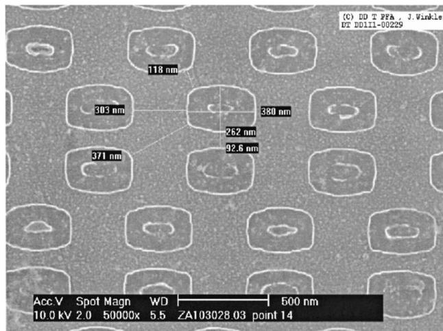
**Figure 5.** SEM of the asymmetric storage trench pattern of an actual trench cell-based DRAM product, where COP short fails mainly arise between the most adjacent deep trench pairs, having minimum distances down to 92 nm.
