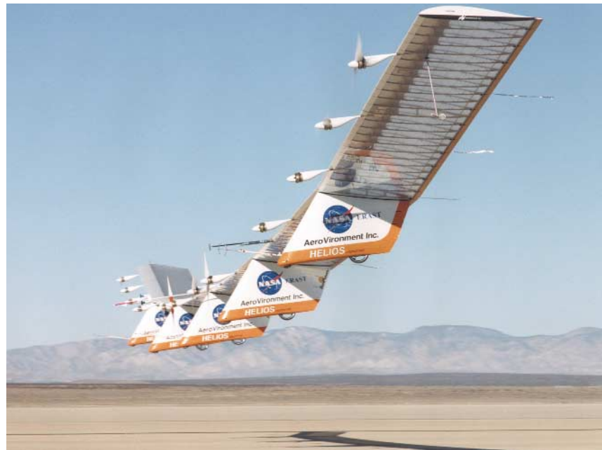
Fig. 6 Helios. AeroVironment's craft has a wing span of 75 m and aims to operate up at 100000ft under solar power (Photo: NASA Dryden/Tom Tschida)
