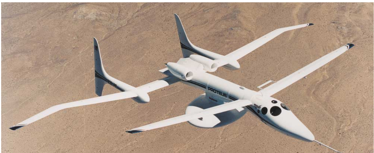
Fig. 7 HALO Proteus aircraft. Note the pod for the payload underneath. (Courtesy of Angel Technologies Corp.)
