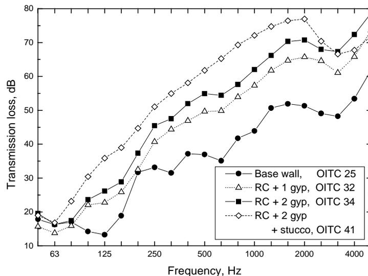
Figure 4. Comparison of results for walls with resilient channels (RC) with the base wall.
