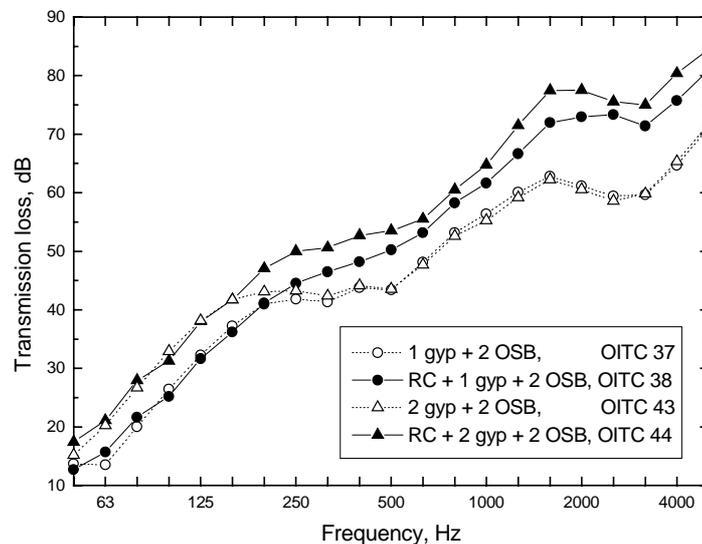
Figure 6. Comparison of results for staggered stud walls with and without resilient channels.
