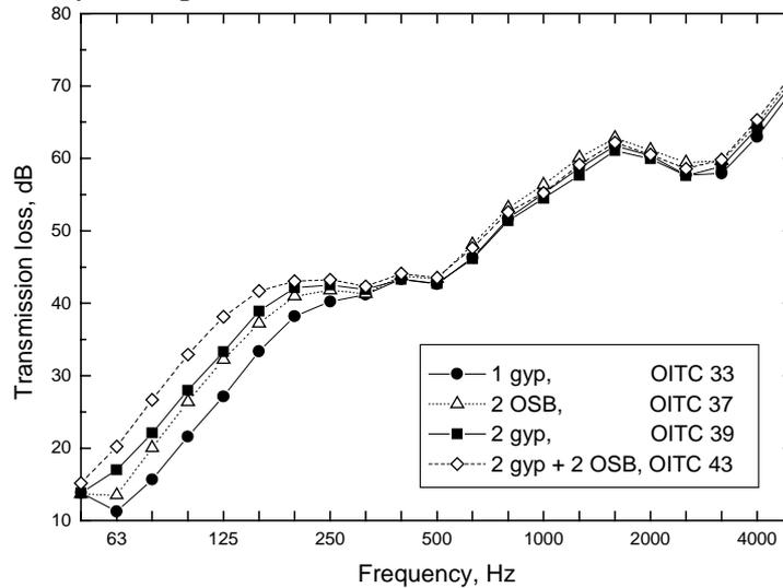
Figure 5. Effects of various surface layers on staggered stud walls.
