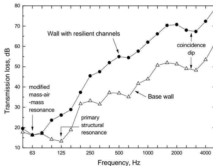
Figure 1. Key characteristics influencing the sound insulation of wood stud walls.
