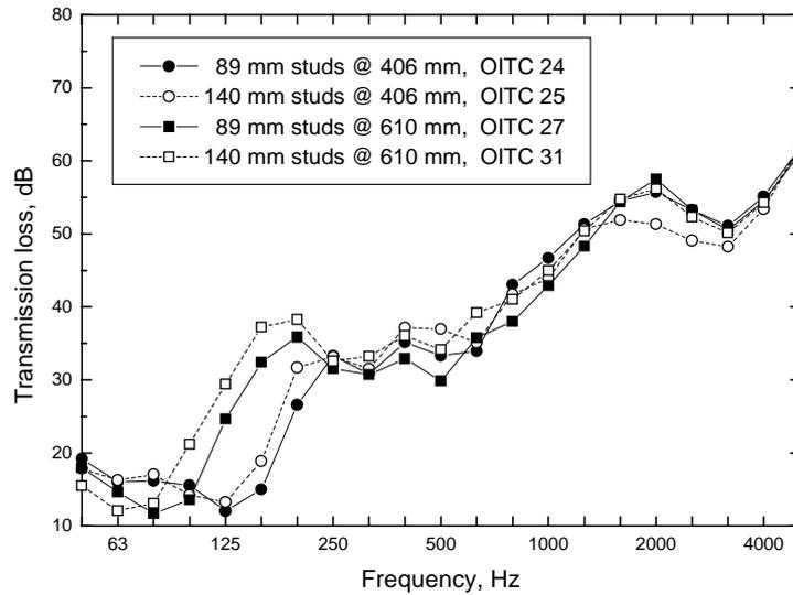
Figure 3. Effects of stud size and stud spacing on measured transmission loss (TL).
