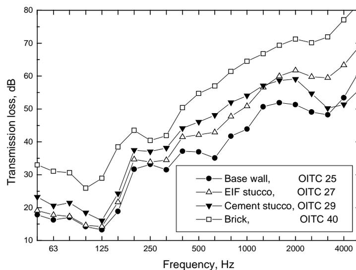
Figure 2. Effects of adding heavier surface layers to the base wall.
