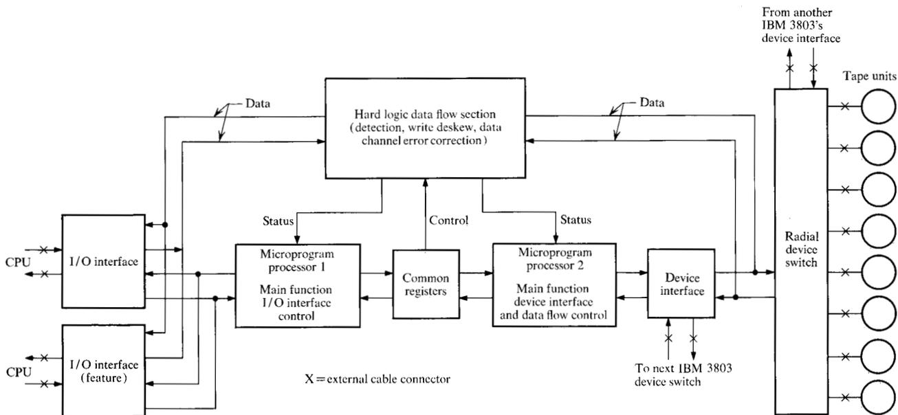
Figure 2 Block diagram of microprocessing.
