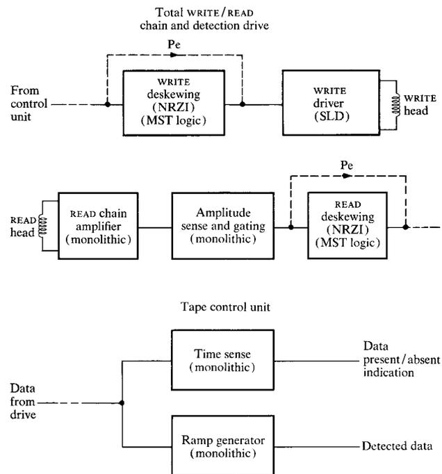
channel diagram, Fig. 10: READ chain, amplitude sense and gating ramp generator, and time sense.
