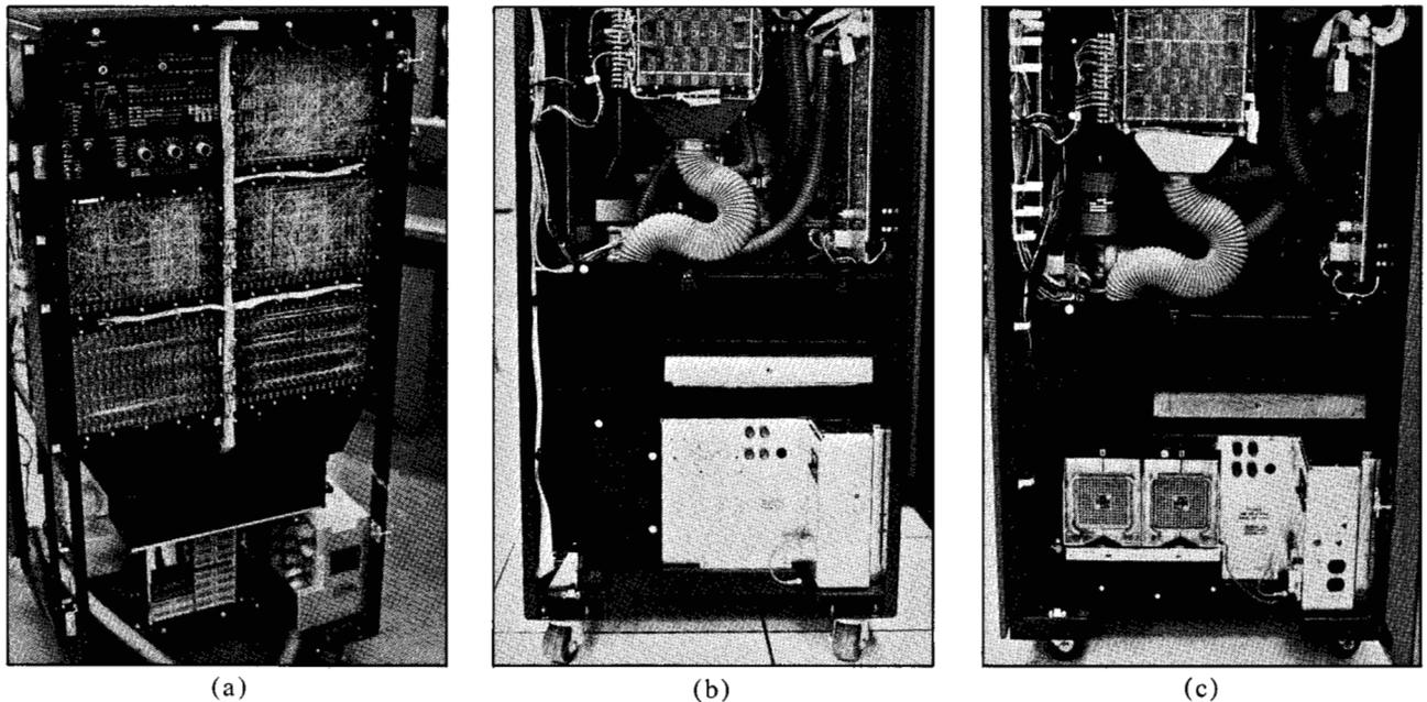
**Figure 3** Tape subsystem packages: (a) Front of IBM 3803 Tape Control Unit, showing CE panel at upper left; (b) Rear of IBM 3420 showing cable connector at bottom left; (c) Rear of IBM 2420 Magnetic Tape Unit, showing cable connector and power supply at bottom (for comparison).
