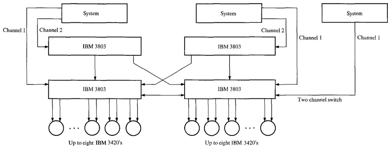
**Figure 1** Configuration of the IBM 3803/3420 Magnetic Tape Subsystem showing how four control units communicate with up to 16 tape drives. This example of a typical configuration shows a pool of 3420 drives which can be accessed by three independent systems.
