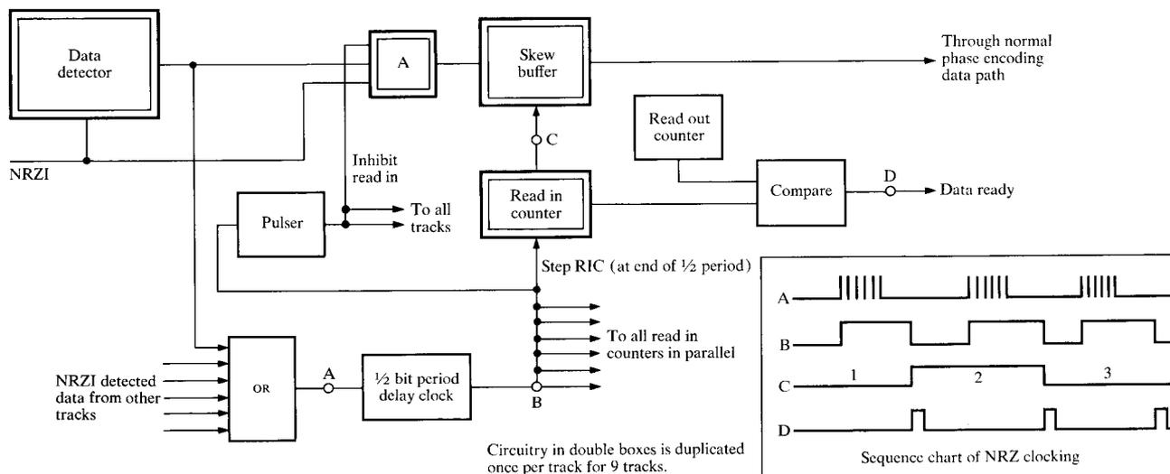
Figure 4 NRZ detection with conversion of NRZ to pseudo-phase encoding.
