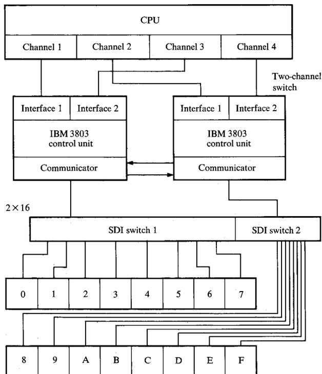
Figure 5 Typical two-channel switch system including 16 tape drives attached.
