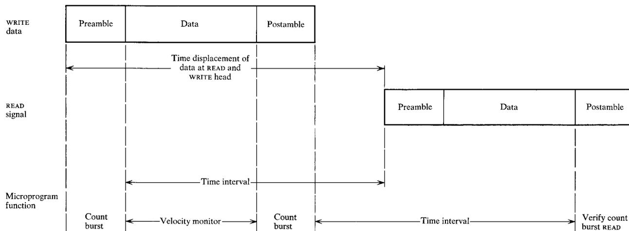
Figure 8 Microprogramming monitor of WRITE data format.
