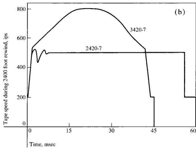
Figure 9 Tape velocity data. (a) Reel speed during worst-case capstan reversals. (b) Rewind speed characteristics.
