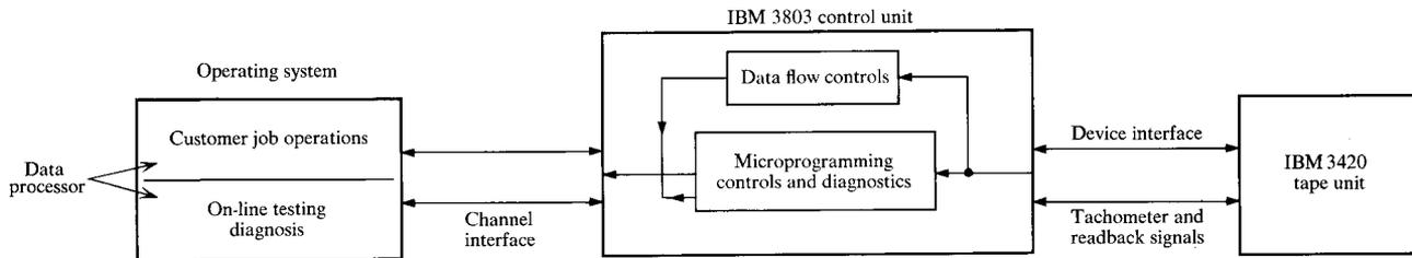
Figure 6 The on-line diagnostic function of the IBM 3803/3420 Magnetic Tape Subsystem.
