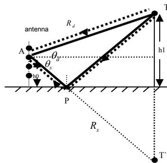
Figure 2. MIMO radar signal of multipath transceiver co-located element linear array model
