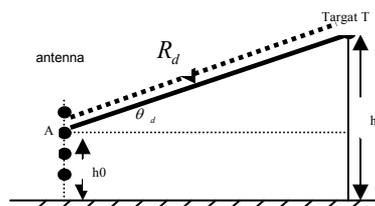
Figure 1. The co-location transceiver element linear array MIMO radar signal model
