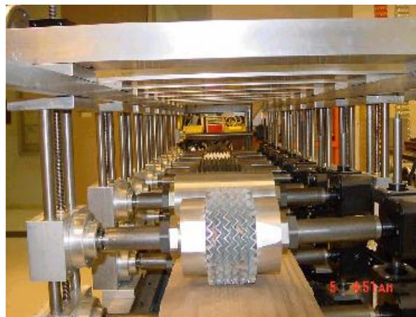
**Figure 13** Photograph of sheet folding rolling sequence
