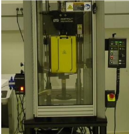
**Figure 15.** Head of the INSTRON Impact Testing Machine With Added Weight Compartment
