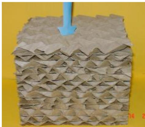
**Figure 16.** Flat Orientation of Folded Chevron Pad With Arrow Showing Direction of the Impacted Force
