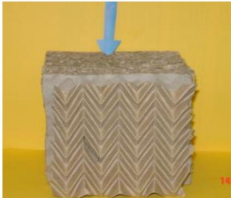
**Figure 18.** Vertical Orientation of Folded Chevron Pad With Arrow Showing Direction of the Impacted Force
