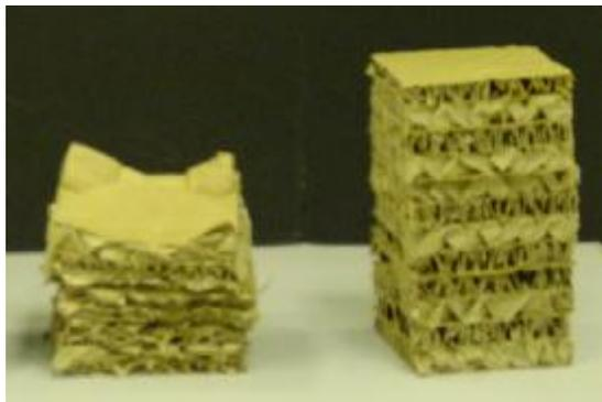
**Figure 23.** Folded Sample Before and After Impact
