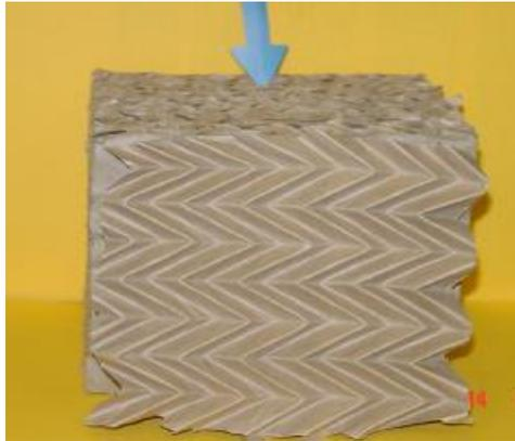
**Figure 17.** Side Orientation of Folded Chevron Pad With Arrow Showing Direction of the Impacted Force
