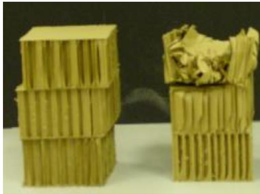
**Figure 24.** Honeycomb samples before and after impact
