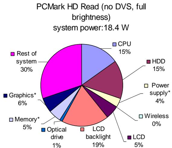
Figure 5: Breakdown of power consumption under different PCMark2002 benchmarks
