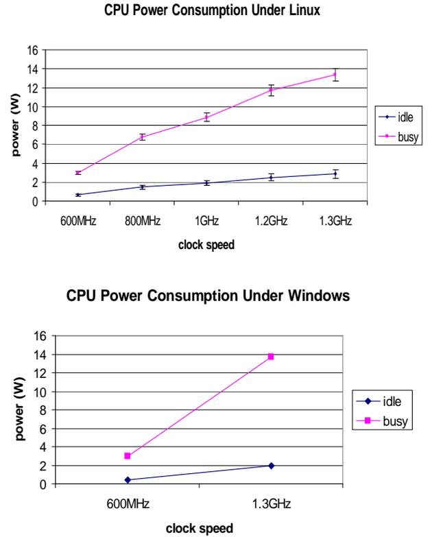
**Figure 2: CPU power consumption under Linux and Windows using calculated  $\alpha C$ .**
