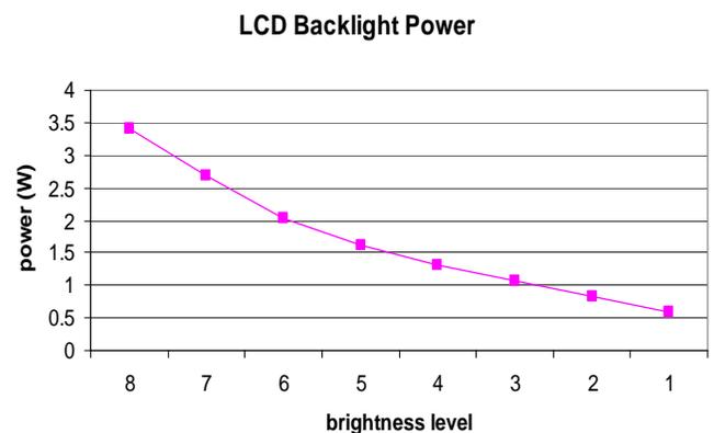
**Figure 1: Backlight power versus brightness level**
