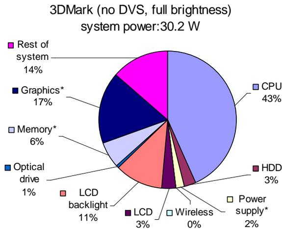
**Figure 8: Power consumption breakdown of 3DMark01**
