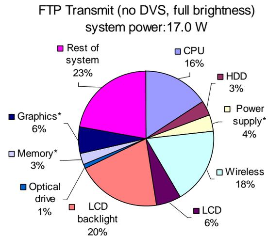
Figure 6: Power consumption breakdown of FTP
