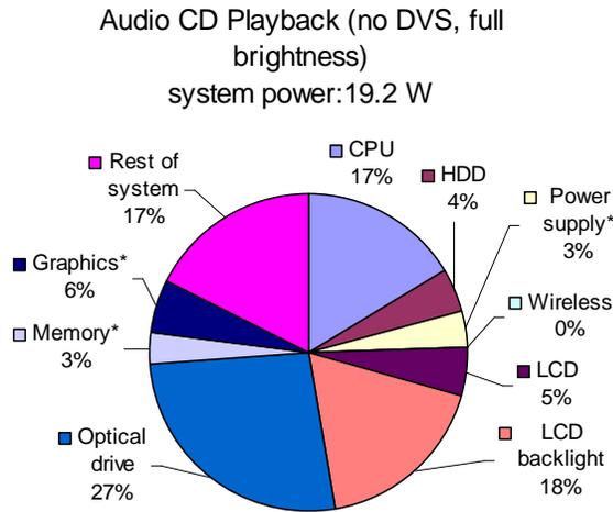
**Figure 7: Power consumption breakdown of audio CD playback**
