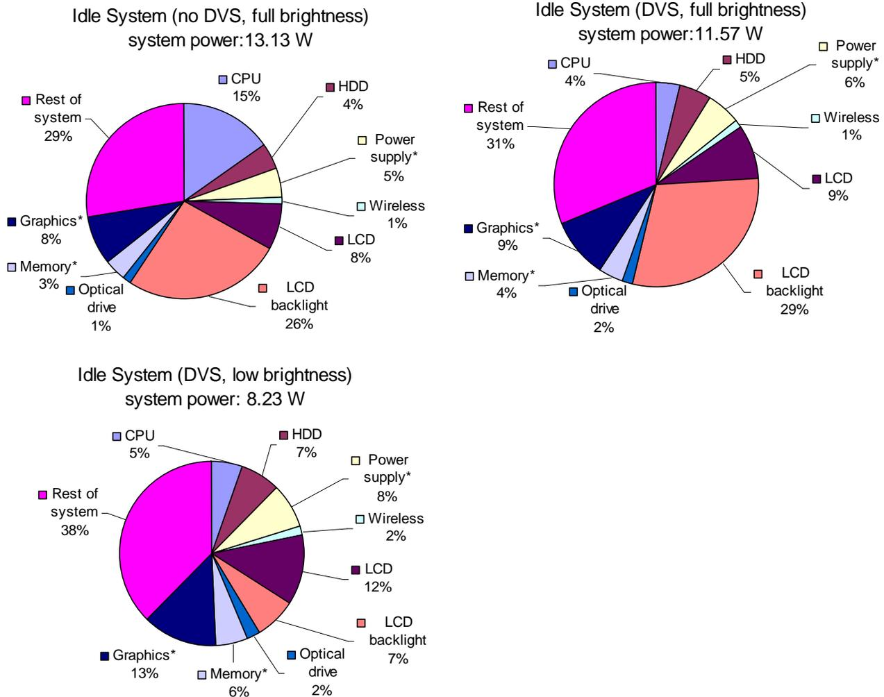
Figure 4: Breakdown of idle system power conversion with various CPU speeds and display brightness levels
