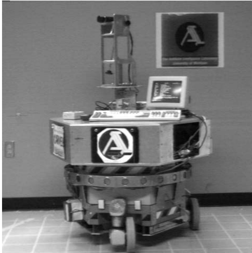
Figure 1: CARMEL stands just under a meter tall and moves at speeds up to 780 mm/sec. A ring of 24 sonars surrounds the robot's torso; a grayscale CCD camera mounted on a rotating tower provides visual capabilities. The monitor and keyboard are used for debugging, and not used in actual competition.
