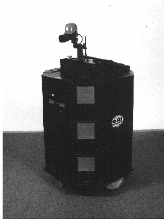
Figure 2: Flakey is about one meter high and moves at speeds up to 500 mm/sec. Twelve sonars (four in front, four in back, and 2 at each side), and eight touch-sensitive bumpers surround the robot. A structured-light sensor provides a dense depth map over a small region in front of Flakey.
