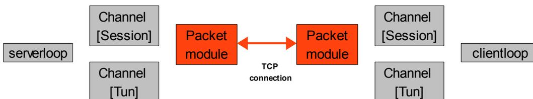
**Figure 8:** The important modules involved in the communication between server and client. The packet module is in red to indicate that encryption is taking place and the connection to the client is thus encrypted when the VPN connection is initialized.
