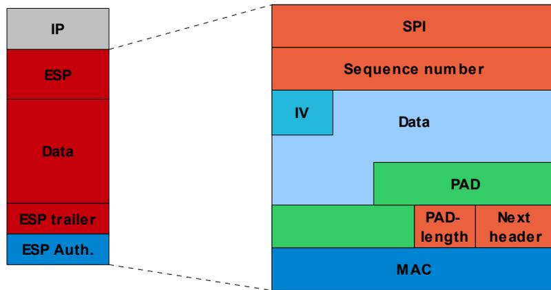
**Figure 4:** To the left, an IP datagram containing an ESP header. To the right, the fields in an ESP header including an IV for the cipher.
