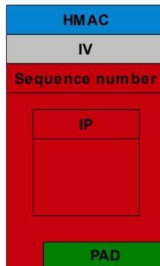
**Figure 6:** An OpenVPN packet containing a tunneled IP packet.
