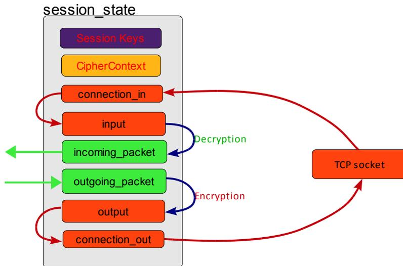
**Figure 9:** The session state data structure maintaining the state of the packet module. The arrows indicate the data flow, in the VPN case containing IP packets, between the objects. Green colour denotes unencrypted data, red denotes encrypted data and blue denotes data being encrypted or decrypted.
