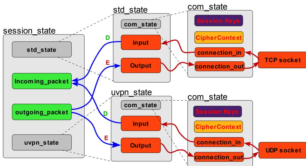
*Figure 11: The organization of the new session state structure, located in packet.c, and its sub structures. Red color indicates encrypted data. Green indicates unencrypted data.*
