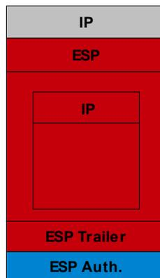
**Figure 5:** A tunnelled IP packet when using a tunnel mode SA and ESP.
