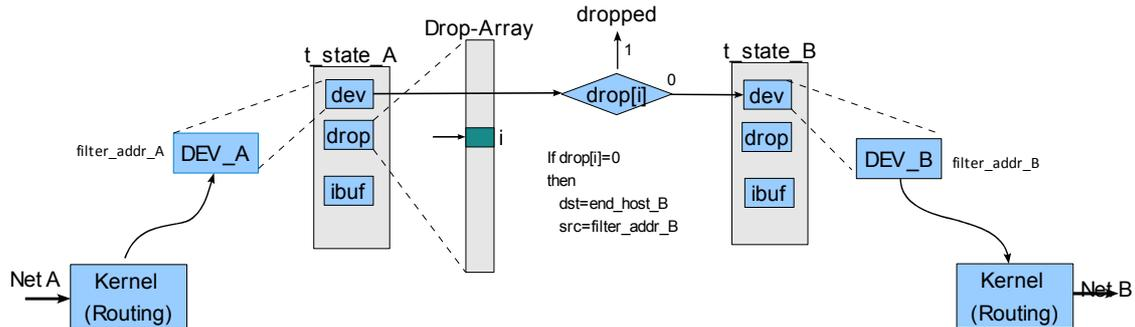
**Figure 17:** Filtering of packets, by *spf*, going from Network A to Network B.
