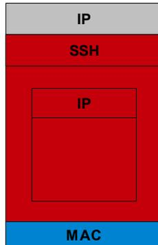
**Figure 3:** A tunnelled IP packet in an SSH packet. Red denoting encrypted information.
