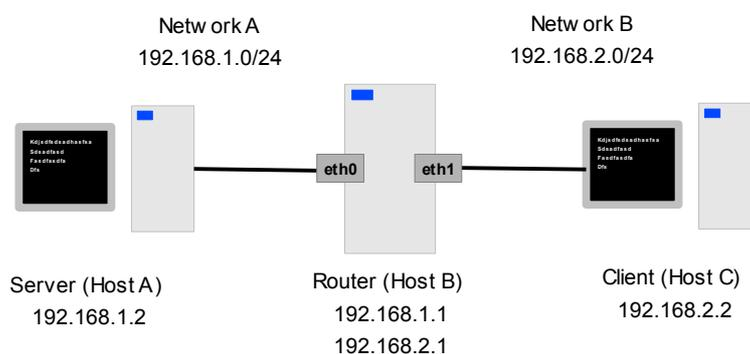
**Figure 16:** The test bench, showing the Server host, the Router host and the Client host.
