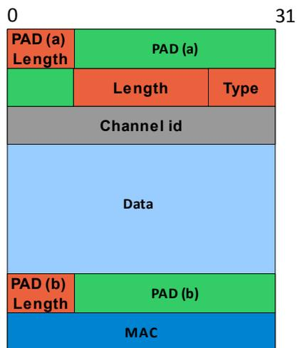
*Figure 15: The modified SSH packet in order to avoid predictability. The PAD divided into part a and part b which are preceded with length fields.*
