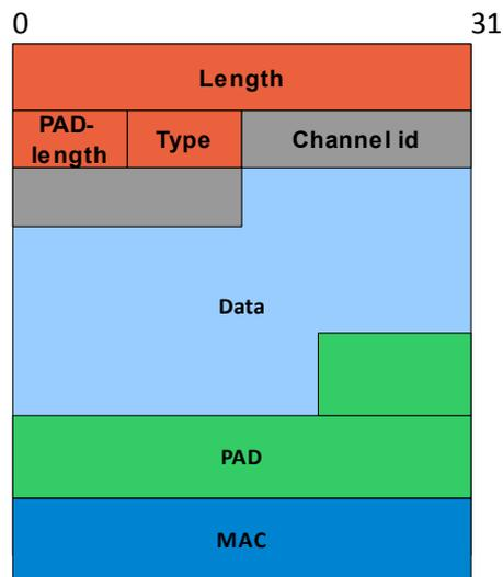
*Figure 2: SSH packet used to send data for a logical channel.*
