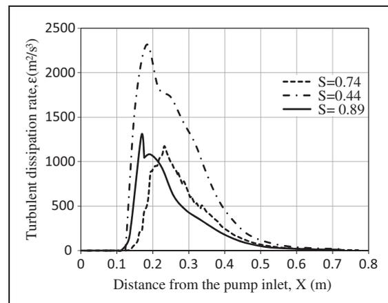
**Figure 8.** Dissipation rates of the turbulent kinetic energy along the jet pump centerline for the driving nozzle positions at optimum flow ratios ( $A = 7.94$  and  $L = 7.4$ ).
