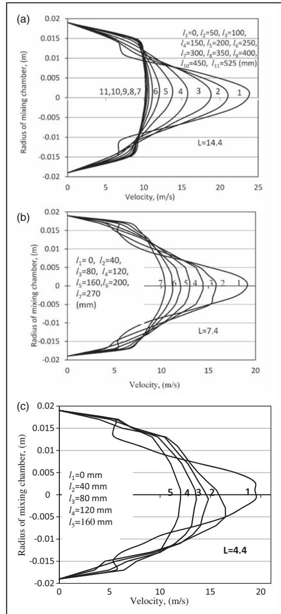
**Figure 6.** Velocity profiles of flow within the mixing chamber: (a)  $L = 14.4$ , (b)  $L = 7.4$ , and (c)  $L = 4.4$ .
