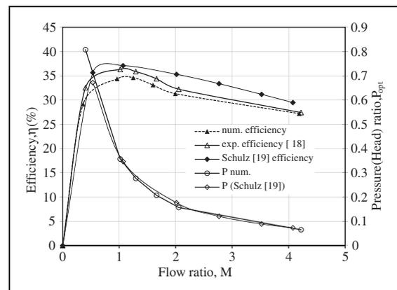
Figure 10. The numerical and experimental optimum curves.
