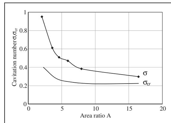
Figure 13. Cavitation numbers at the optimum operating conditions.
