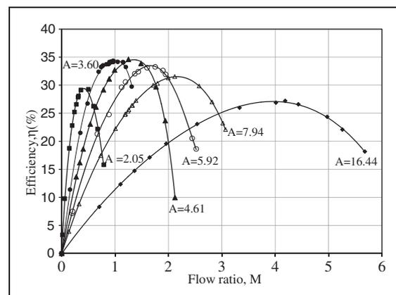
**Figure 9.** Numerical efficiency curves at various area ratios.
