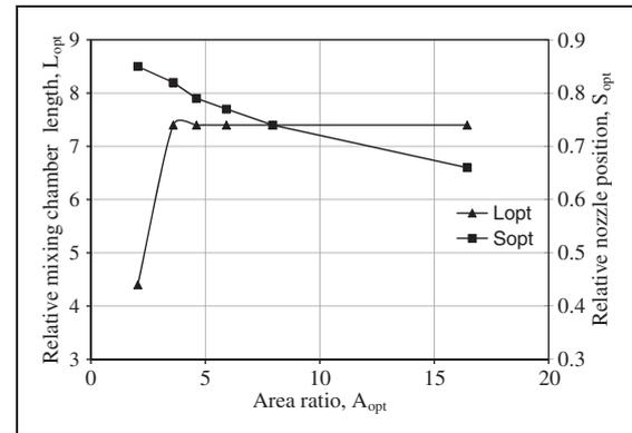
Figure 12. Optimum relative nozzle position  $S_{opt}$  and mixing chamber length  $L_{opt}$ .
