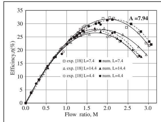
**Figure 4.** Effect of the mixing chamber length on the efficiency.
