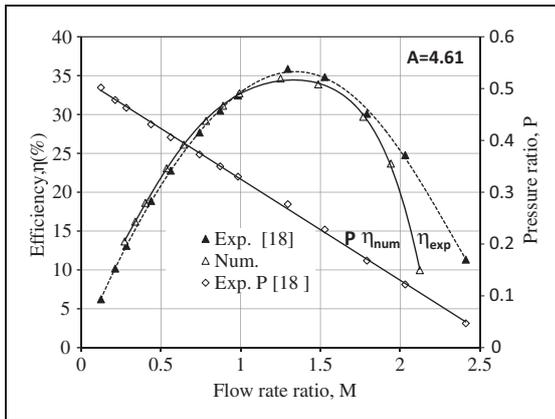
**Figure 3.** The numerical and experimental performance curves at constant area ratio.
