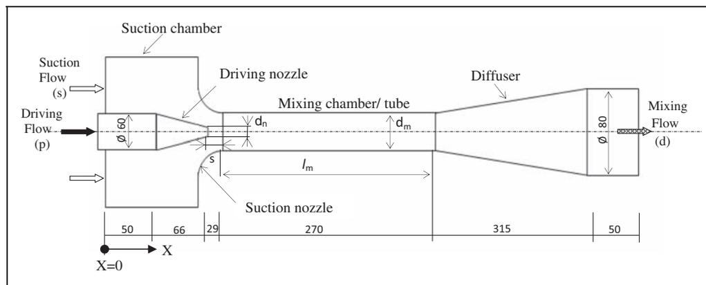
Figure 1. Schematic of the computational domain.
