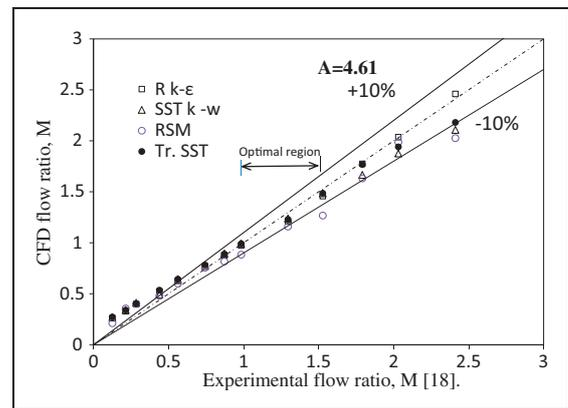
**Figure 2.** CFD results versus experimental flow ratios.
