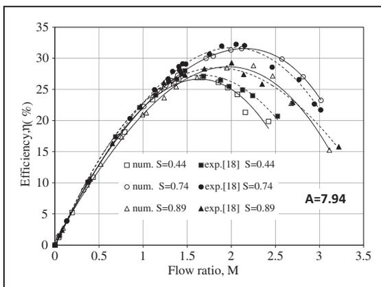
**Figure 7.** Effect of driving nozzle position on the efficiency of the pump.
