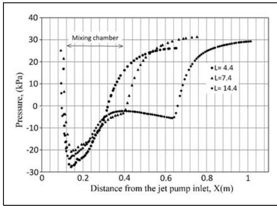
**Figure 5.** Pressure variations on the jet pump centerline.
