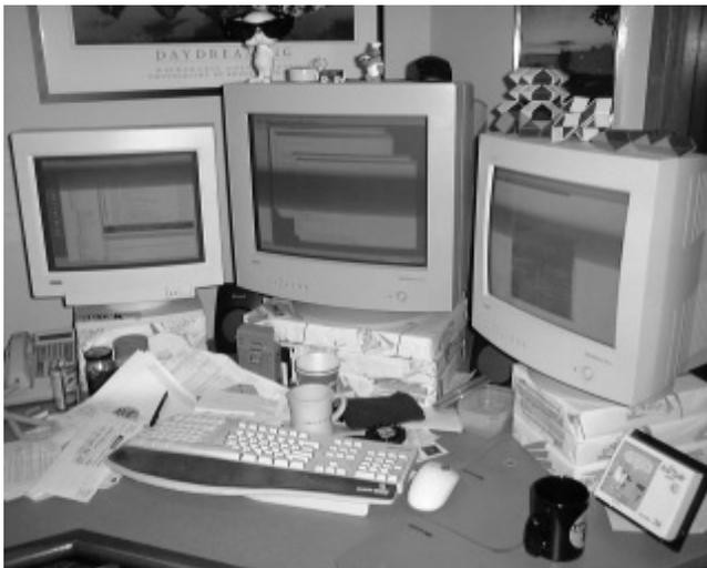
**Figure 2. A 3-monitor configuration. Displays are not pushed as close together as possible to minimize gaps.**
