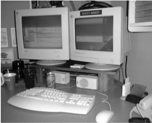
**Figure 1. A 2-monitor configuration. Note bezels interrupting the display surface.**
