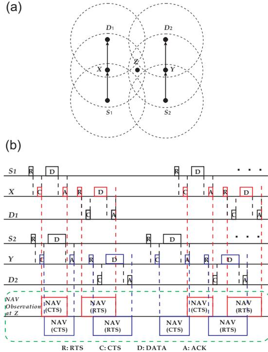
**Figure 1.** Schematic diagrams of (a) an exemplified network topology and (b) the RTS/CTS-based collision avoidance scheme associated with the NAV vectors.
