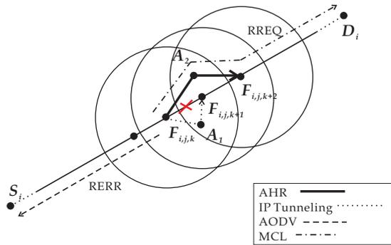
**Figure 2.** Schematic diagram for the route repair schemes.
