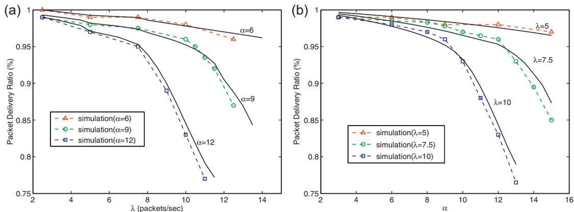
Figure 6. (a) Packet delivery ratio versus data rate  $\lambda$ ; (b) Packet delivery ratio versus number of interfering neighbors  $\alpha$  (Solid lines: analytical results; Dashed lines: simulation results).
