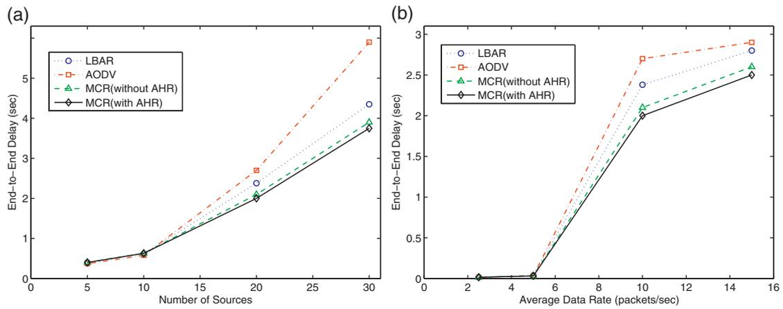
**Figure 12.** Simulation results of the random topology: (a) Average end-to-end delay *versus* number of sources; (b) Average end-to-end delay *versus* average data rate.
