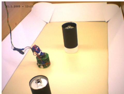
Fig. 3. The robot sits pensively in its arena. The cylinders are soft-drink cans wrapped in black paper. The camera on top of the robot images a horizontal line of 64 grey-scale pixels spanning 36 degrees.
