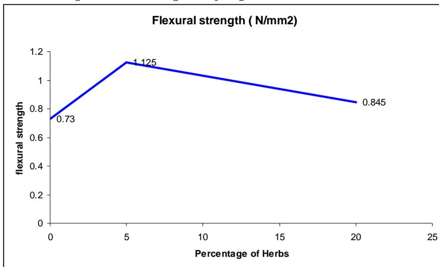
The flexure strength of lime and herbal mortar are tabulated in Table 2. The flexure strength of lime mortar is 0.703 N/ mm<sup>2</sup>. As shown in the Fig.1, the transverse strength is maximum for 5% herbs (1.125N/ mm<sup>2</sup>) which is 1.6 times greater than that of plain lime mortar. However, there is an increase of flexure by around 20% for 20% of herbs. Therefore for a better flexibility 5% herbs can be added with the lime mortar (5%
