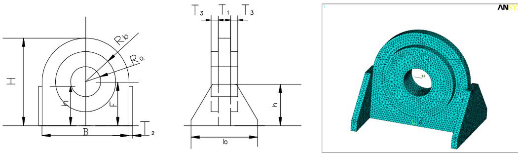
Fig.1 The structural forms and FEM model of D padeye
