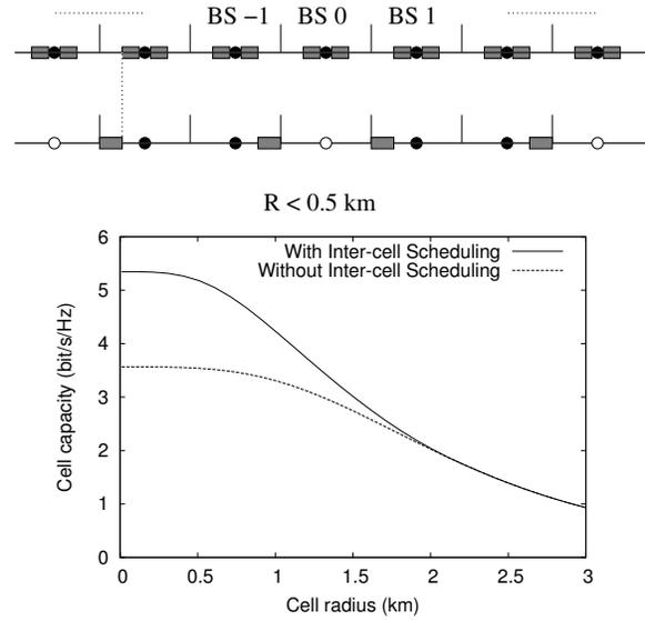
Figure 4: Optimal static scheduling strategy (left) and capacity (right) of a linear network.
