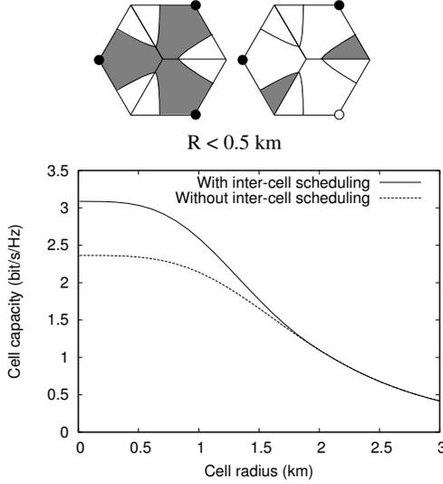
Figure 3: Optimal static scheduling strategy (left) and capacity (right) of a tri-sectorized hexagonal network.
