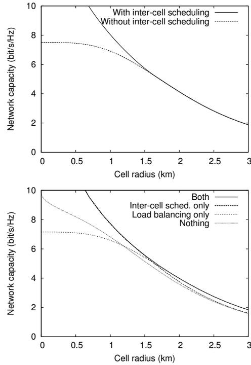
Figure 2: Capacity of a two-cell symmetric (left) or asymmetric (right) network.
