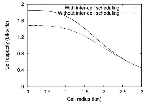
Figure 7: Capacity of a hexagonal network.
