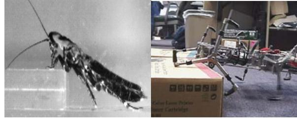
Figure 5. Like the cockroach, Whegs brings its legs into phase to climb obstacles.
