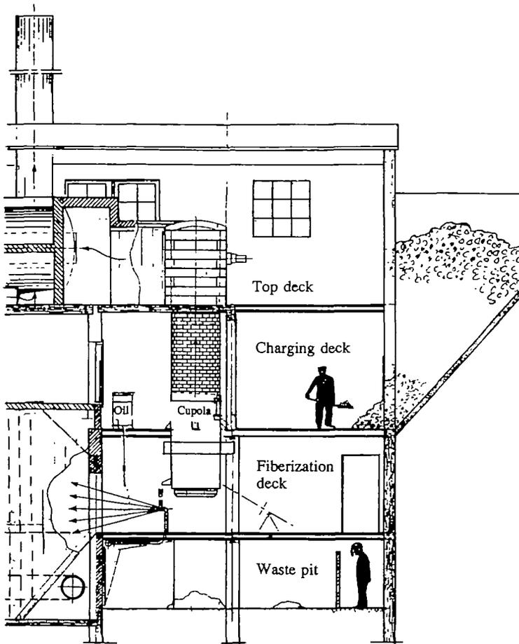
FIG. 1. Cupola furnace and furnace house.
