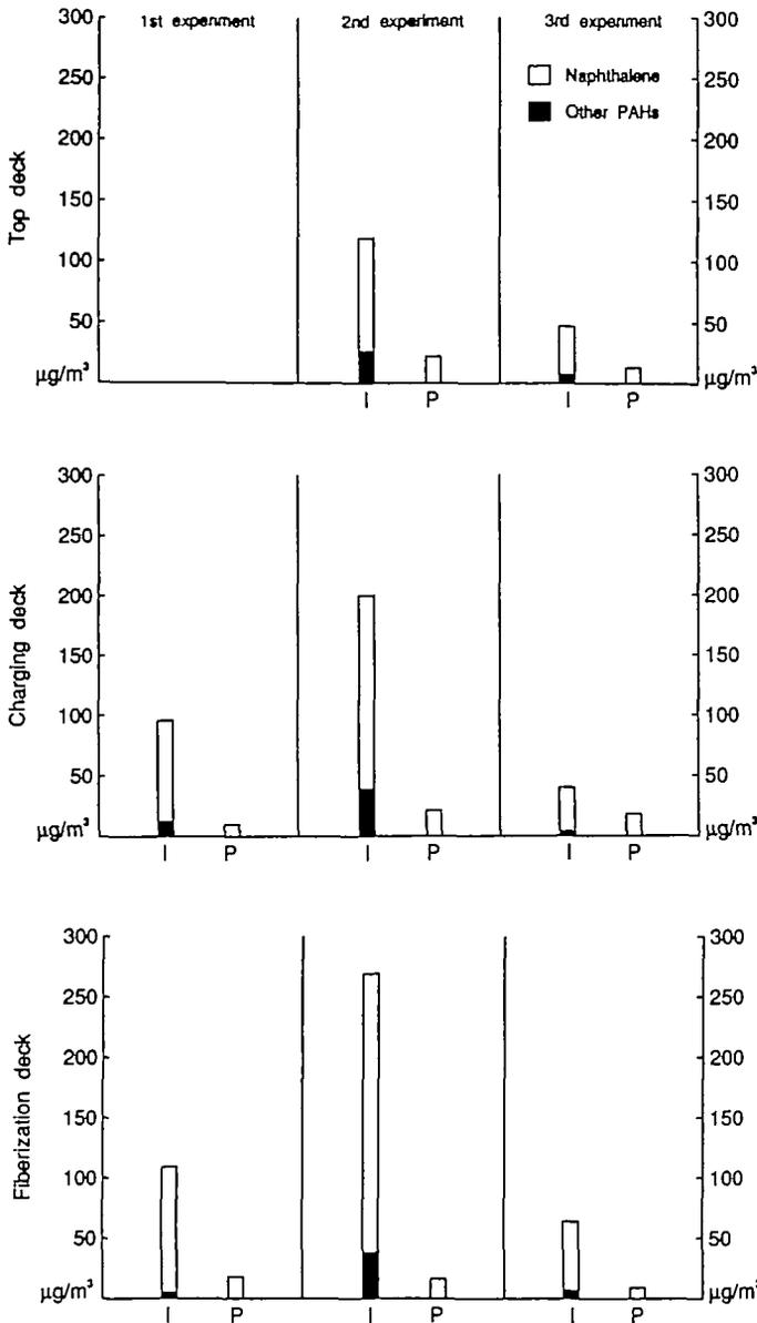
FIG. 2. Concentrations of PAHs during the ignition phase (I) and during normal production (P).
