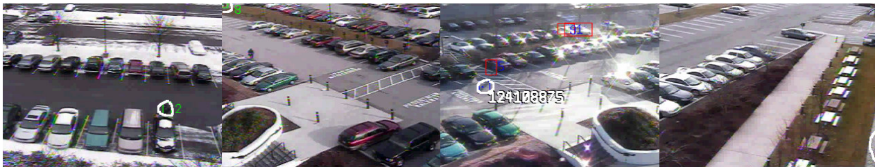
Figure 6. Two pictures on left are example frames from track FNs - the first is not detected because of insufficient contrast, the second because it lies on the border of the video image (upper left). Two pictures on right are examples from track FPs – the first is the result of significant shadows, the second from reflections off glass of building (bottom right of image.)
