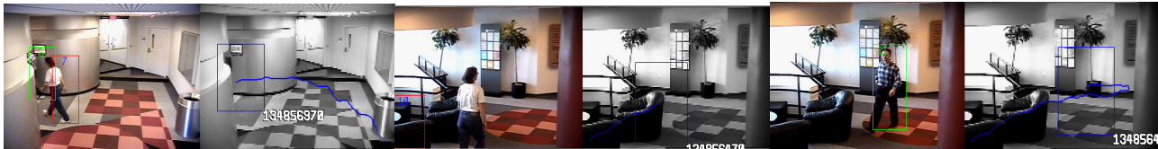
Figure 7. Left two images: spatial merge – system combines two people into one track, Middle two images: 1 st person walks across, Last two images: 2 nd person then walks, causing temporal merge – system combines tracks of both people, one after the other.
