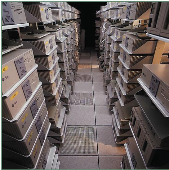
Figure 4. 100-node 200-CPU cluster. Key design points include extreme symmetry, internal disks, no people, no monitors, and no visible cables.
