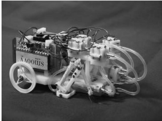
**Figure 6. Small hybrid wheel-leg robot**
