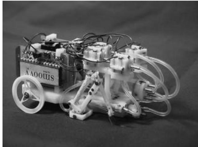
**Figure 6. Small hybrid wheel-leg robot**
