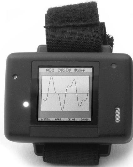
Fig. 4. A photo of the wrist unit mechanics ( $72 \times 51 \times 22$  mm).
