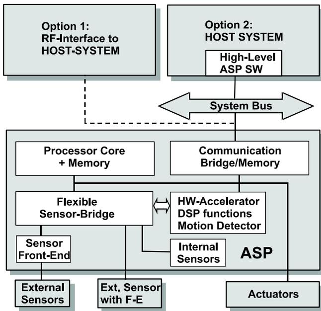
Fig. 1. The ASP architecture. The ASP can interface to the application processor via a wireless radio (Option 1) or via the system bus (Option 2).
