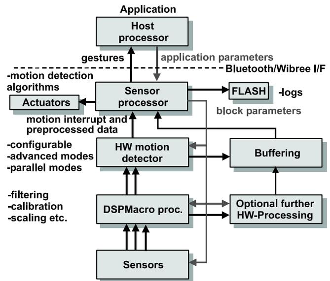
Fig. 2. An example of power efficient accelerometer processing using ASP. Configurable DSP macros process the raw sensor data to reduce data bandwidth. A motion detector implemented in hardware can detect events and alert the processor. Sensor data from these events is optionally further processed by hardware and buffered. Finally the processor does gesture recognition from the data and alerts the application host processor.
