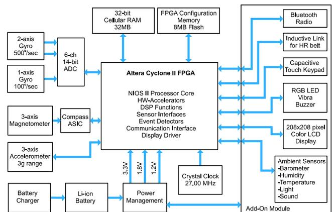
Fig. 3. Diagram of the hardware. The base platform includes the FPGA. Additional sensors, user interface components and wireless connectivity is provided with an add-on module.
