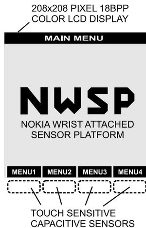
Fig. 5. An example of a user interface for the sensor platform. Below the LCD display there are four capacitive sensors that are touch sensitive.
