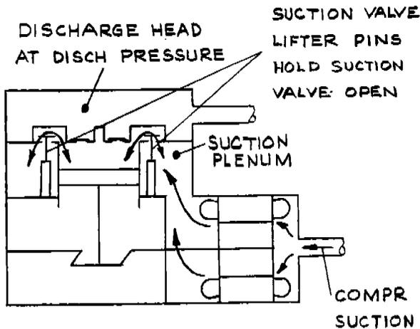
FIGURE 4. SUCTION VALVE LIFTER UNLOADING SHOWN UNLOADED
