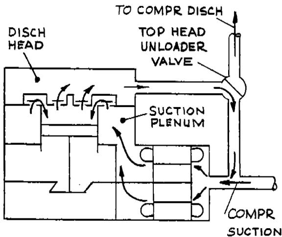
FIGURE 1. TOP HEAD UNLOADING, (THU) SHOWN UNLOADED TO COMPRESSOR SUCTION
