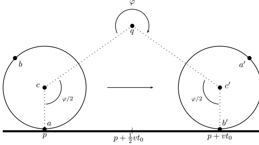
Figure 2: This shows the starting and stopping position of a disk which has rolled along the line. The rolling motion is equivalent to rotation by angle  $\varphi$  around the point  $q$ . The points  $a, b$  are fixed points on the circumference of the disk; the point  $c$  is the center of the disk. The positions of the points after the disk has finished rolling are labelled  $a', b', c'$ .
