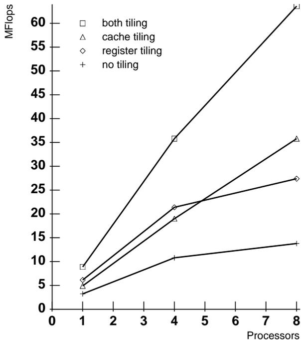
Figure 1: Performance of  $500 \times 500$  double precision matrix multiplication on the SGI 4D/380. Cache tiles are  $64 \times 64$  iterations and register tiles are  $4 \times 2$ .
