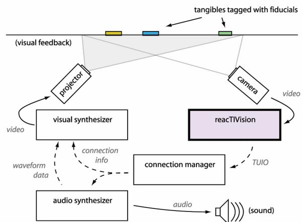
Figure 3. The reacTable components
