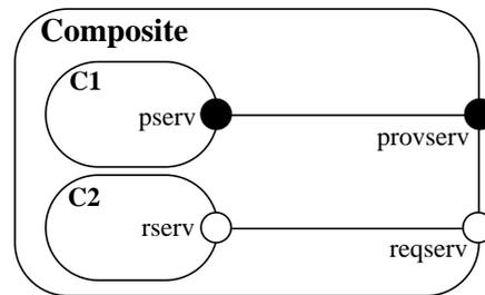
**Fig. 14.** A Darwin composite component. The graphical view of the component is shown on the right. Definitions of basic components C1 and C2, which themselves may be composite, are omitted for simplicity.
