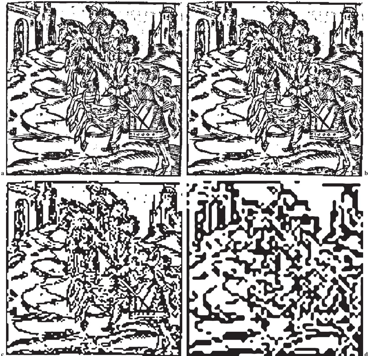
1 Four resolutions of same picture illustrating effect of non-linear median filter ((a) is original image with all detail; (d) keeps only the image main features): (a) binarized original image at resolution 0 ( $512 \times 512$  pixels); (b) resolution 1 ( $256 \times 256$  pixels); (c) resolution 2 ( $128 \times 128$  pixels); (d): resolution 2 ( $64 \times 64$  pixels)
