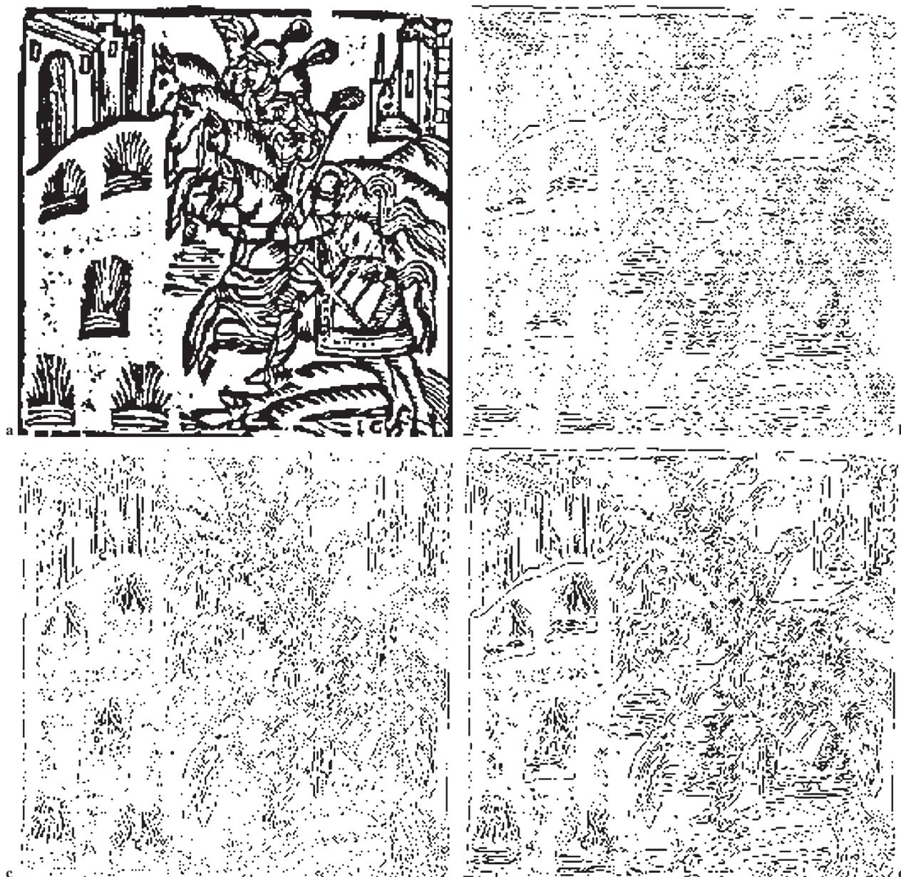
2 Result of non-linear median AMR: approximation 1 and corresponding three detail images: (a) resolution 1 (256 × 256 pixels); (b) vertical detail; (c) horizontal detail; (d) diagonal detail
