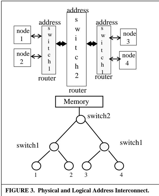
FIGURE 3. Physical and Logical Address Interconnect.
