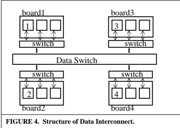
FIGURE 4. Structure of Data Interconnect.
