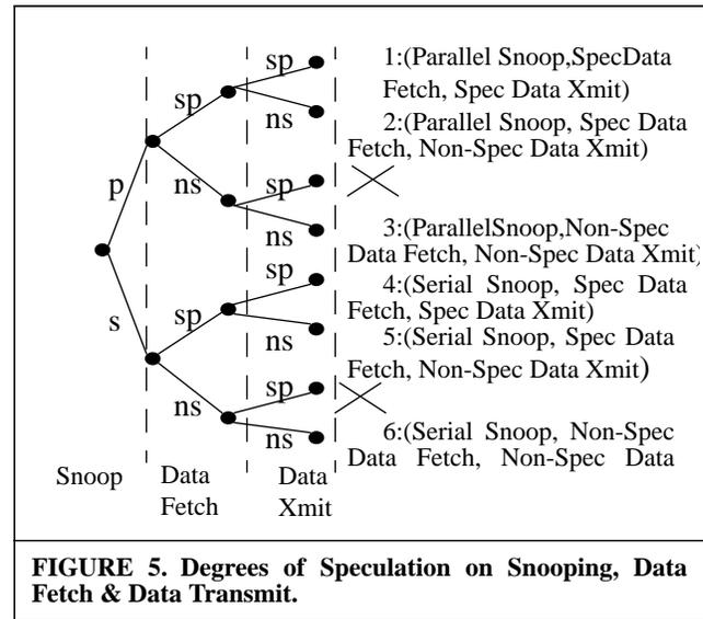
FIGURE 5. Degrees of Speculation on Snooping, Data Fetch & Data Transmit.
