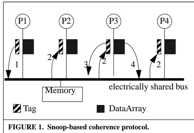
FIGURE 1. Snoop-based coherence protocol.
