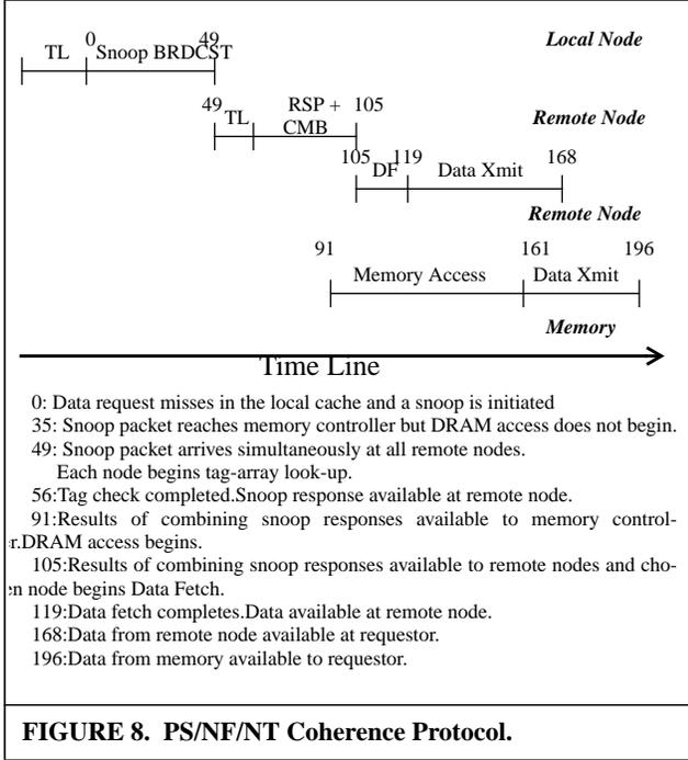
**FIGURE 8. PS/NF/NT Coherence Protocol.**
