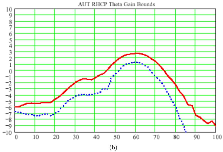
Figure 1.7. Maximum and minimum gain at 7.2 GHz for antennas (a) ST5-3-10; (b) QFH.
