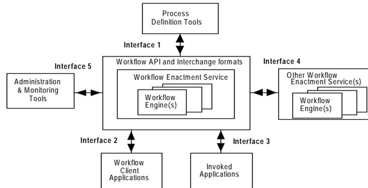
Figure 14. Workflow Reference Model - Interfaces
