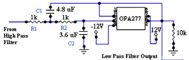
Fig. 7 2<sup>nd</sup> order Bessel's low pass filter
