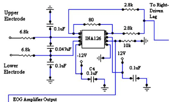
Fig. 3 INA126 with RFI and ESI protection system
