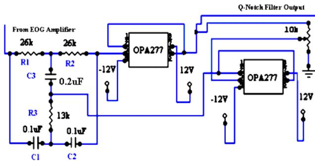
Fig. 5 Q-notch filter
