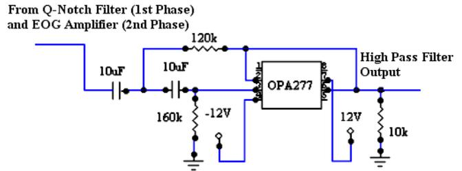
Fig. 6 2<sup>nd</sup> order Bessel's high pass filter
