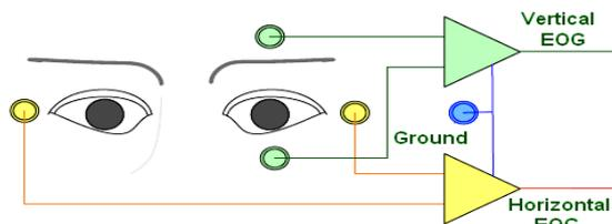
Fig. 2 Correct positions of five electrodes [8]
