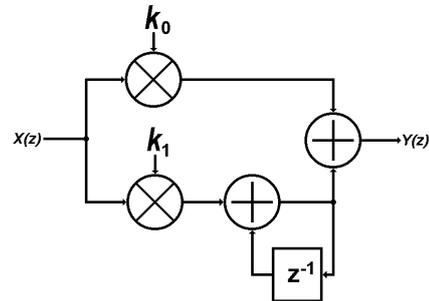
Fig. 3 Block diagram of loop filter for 2<sup>nd</sup> order DPLL
