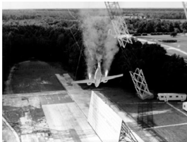
Figure 5. Photograph of a full-scale crash test of a Piper Navajo aircraft with VAS.
