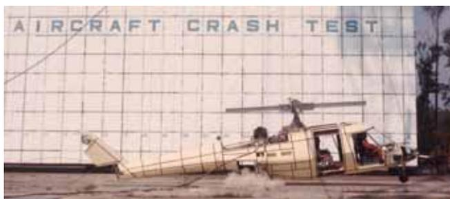
(c) Photograph of the Sikorsky ACAP helicopter during full-scale crash test.
