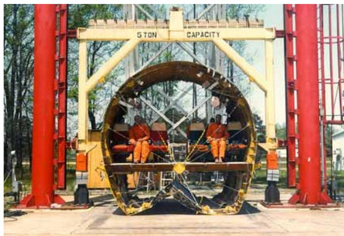
Figure 12. Photograph of the B707 forward fuselage section post-test.
