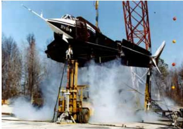
Figure 14. Tethered-hover test of the XFV-12A in 1978.
