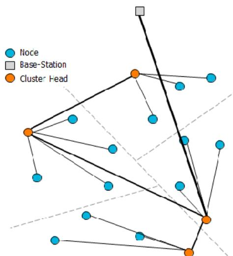
Fig 2: BCDCP protocol after Setup and Data Communication Phase
