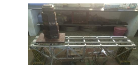
Fig.4: A close view of bridge loaded at center, 200mm offset and 400mm offset in damaged condition
