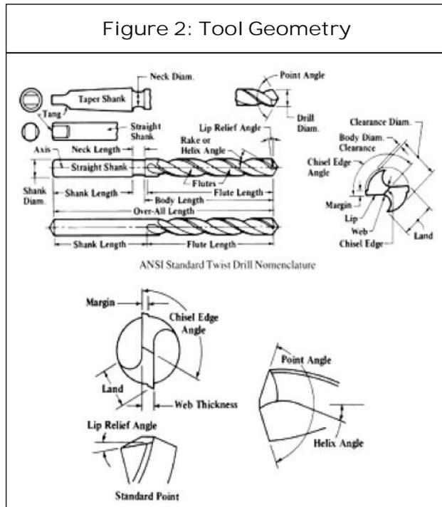
bit is used in high feed rate applications under low spindle speeds, where removal of a large volume of swarf is required. Low spiral (low twist rate or “elongated flute”) drill bits are used in cutting applications where high cutting speeds are traditionally used, and where the material has a tendency to gall on the bit or otherwise clog the hole, such as aluminum or copper.
