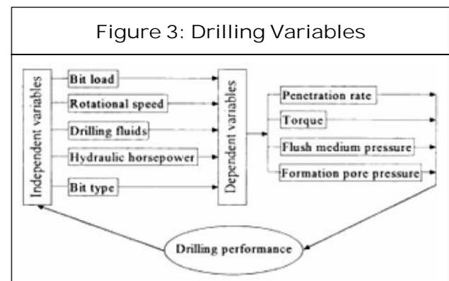
**Dependent Variables:** The dependent variables associated with rotary drilling represent the response of the drilling system to the imposed conditions and are the penetration rate of the bit, the torque and the flush medium pressure.
