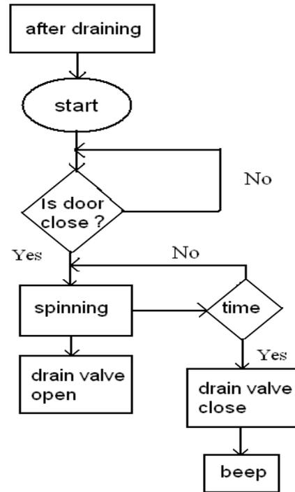
Fig. 4. Flowchart of drying module
