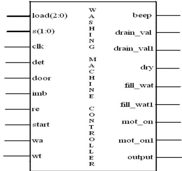
Fig. 5. RTL view of washing machine controller
