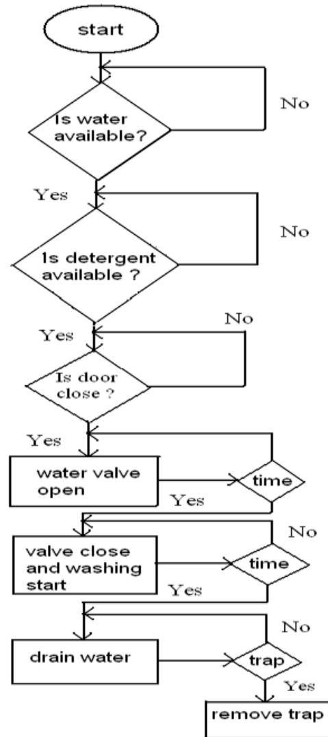
Fig. 2. Flowchart of washing module
