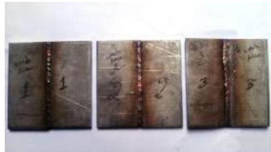
**Fig. 1.2 Welded Samples 304 Stainless Steel**
