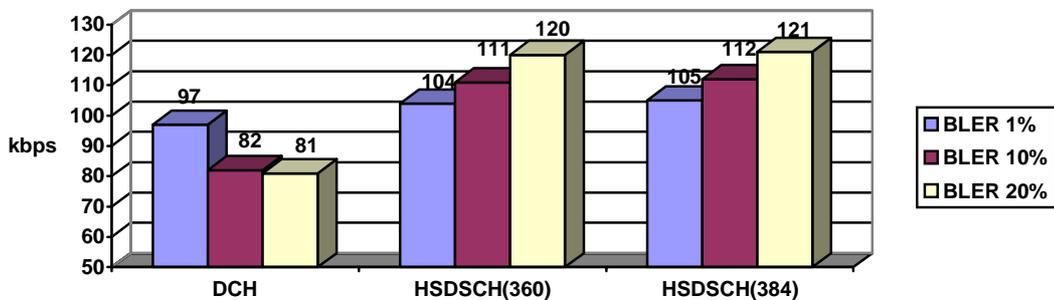
Figure 15. Retransmit Bit Rates with a file size of 20k bytes
