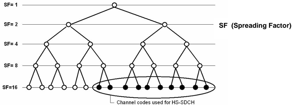
**Figure 4. Multiple codes of spreading factor 16**
