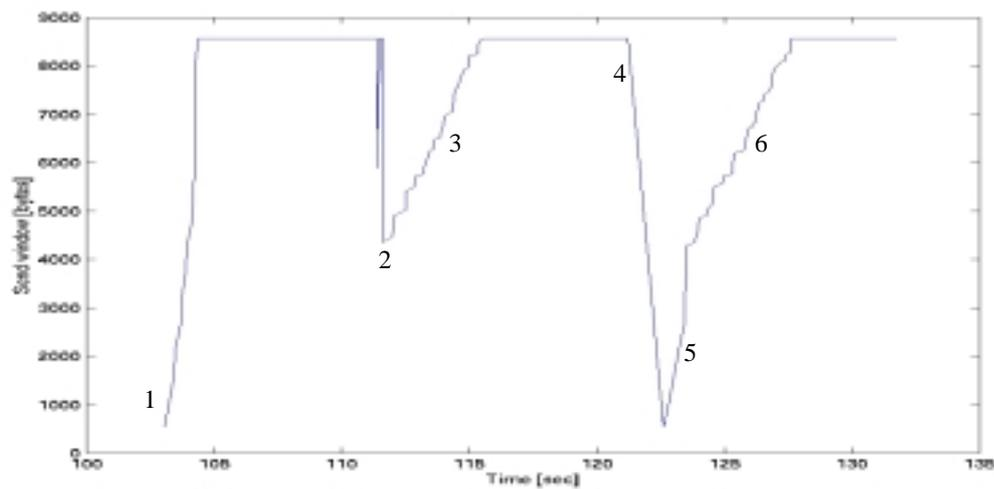
**Figure 1. TCP Send Window, 6 steps: 1. initial slow start; 2. fast retransmission event; 3. congestion avoidance window recovery after a fast retransmission; 4. timeout event; 5. slow start recovery after a timeout; 6. congestion avoidance after the slow start recovery.**
