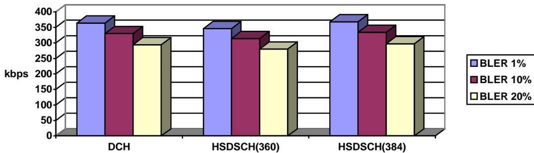
Figure 8. Application Bit Rates with a file size of 16M bytes
