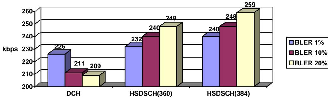
Figure 11. Retransmit Bit Rates with a file size of 100k bytes
