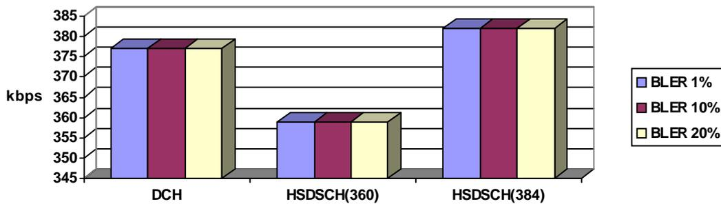
Figure 9. Retransmit Bit Rates with a file size of 16 Mbytes
