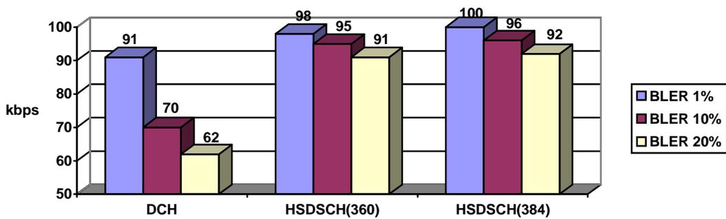
Figure 14. Application Bit Rates with a file size of 20k bytes
