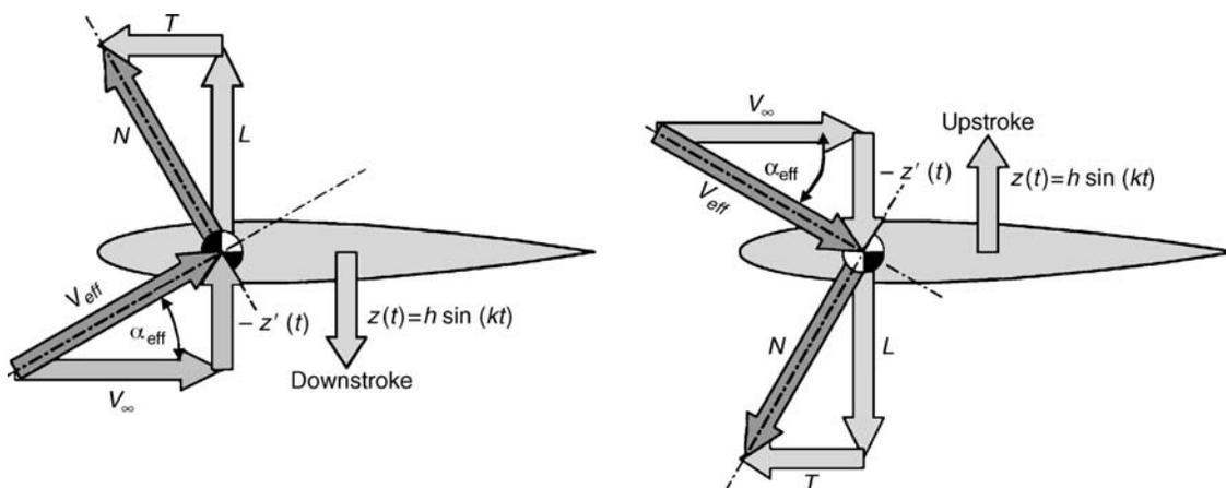
**Figure 3.** Schematic illustrating thrust production by a plunging airfoil as suggested by Knoller (1909) and Betz (1912). Reproduced from Jones and Platzer (2009) © Springer.
