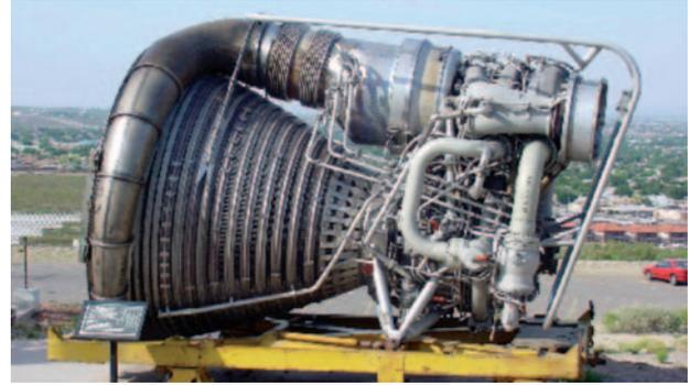
**Figure 8.** An F-1 rocket engine.
