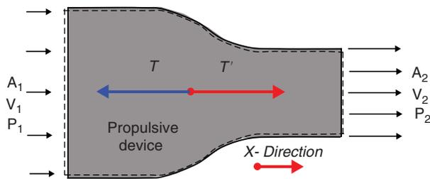
**Figure 9.** Thrust generation by a propulsive device.
