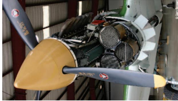
**Figure 5.** An Allison V-1710-115 IC engine-powered propeller.
