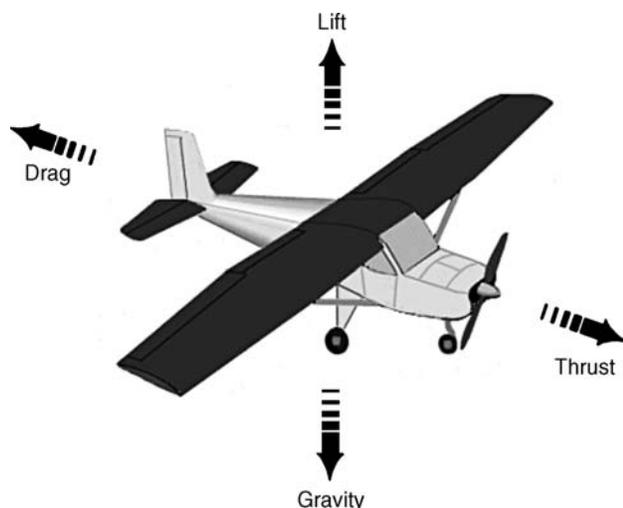
**Figure 1.** The forces that act on an airplane in flight.
