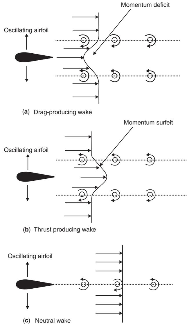
**Figure 4.** Wake structures of an oscillating airfoil.
