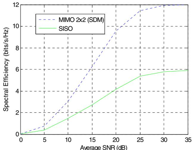
Fig. 6. Spectral Efficiency for SISO and MIMO 2x2 with spatial division multiplexing scheme
