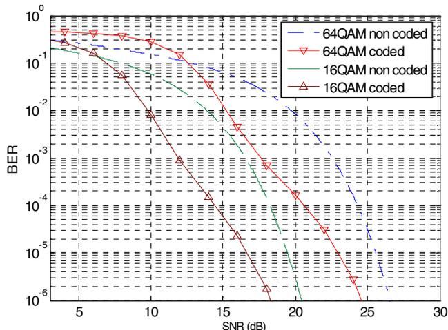
Fig. 5. BER results with and without coding for 16 QAM and 64 QAM.
