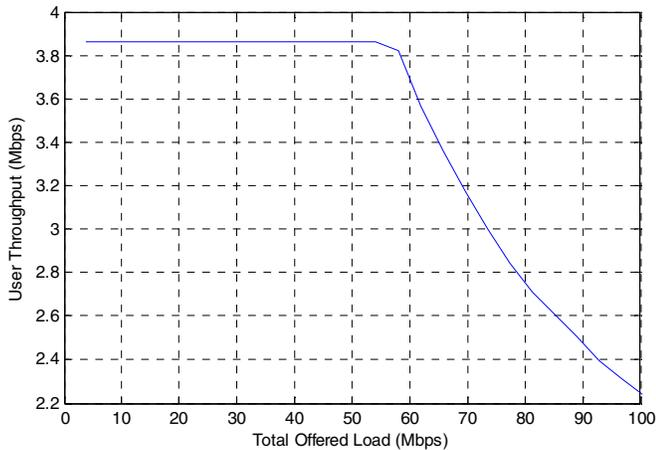
Fig. 7. User Effective Throughput versus Total Offered Load in the system.
