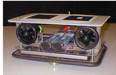
Fig. 1. The MVWT vehicle. A laptop is secured in a Plexiglas chassis that glides on omnidirectional ball casters. Software-controlled high-powered ducted fans attached to the vehicle provide thrust. A MVWT signature on the top the vehicle ( a “hat”) is identified by overhead cameras, and the vehicle receives its position and orientation in a GPS-like fashion over a local wireless network.
