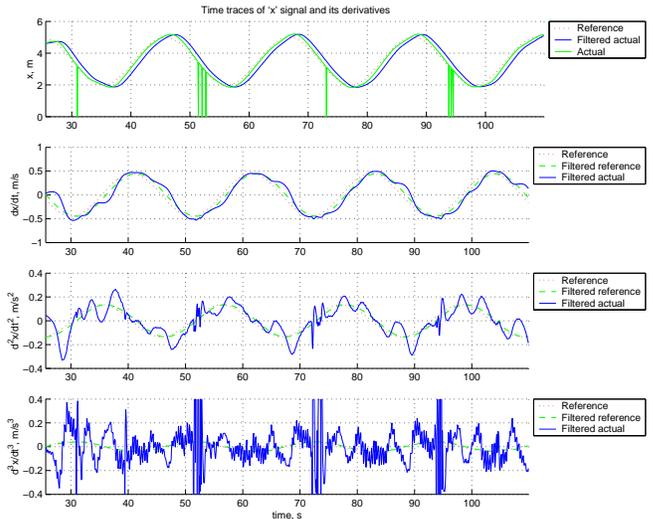
Fig. 5. Time traces of  $x$  position and its first three derivatives for the trajectories in Fig. 4. The reference signals are given by dotted lines and the actual signal by the dash-dotted line in the first plot. The filter outputs, given the actual data as input, are shown by solid lines.
