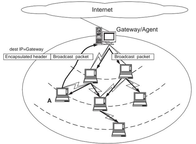
Fig. 5. Routing scenario of broadcasting.
