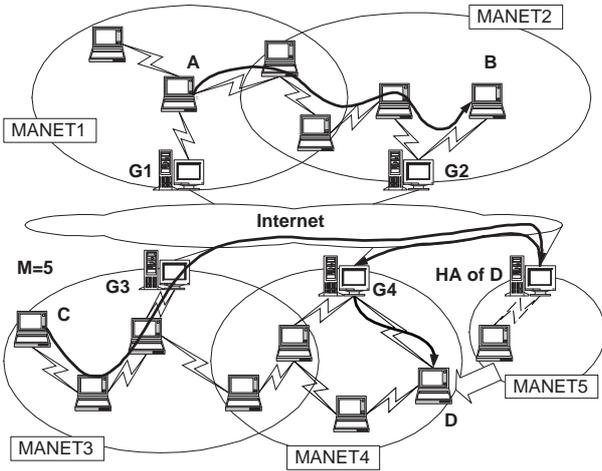
Fig. 4. Inter-MANET routing scenarios in overlaid MANETs.
