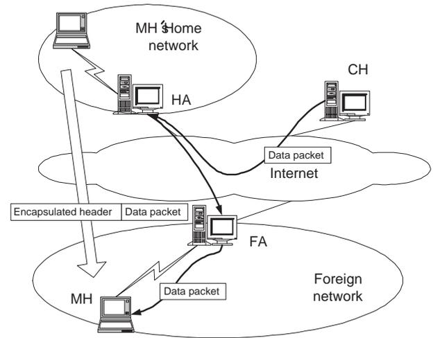
Fig. 1. The transmission scenario of Mobile IP.
