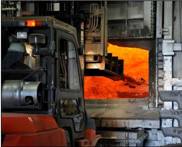
**FIGURE 4 – Worker skimming molten aluminum during the manufacturing process.**
