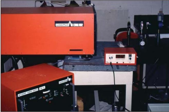
**Figure 3.** The first experimental excimer laser used in performing cadaver eye and animal experiments at Columbia University 25 years ago. Note the power supply (lower device) and laser cavity (upper device).
