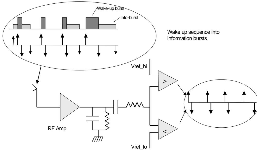
Figure 12.3.3. Reactive radio combines wake-up sequence with information bursts.
