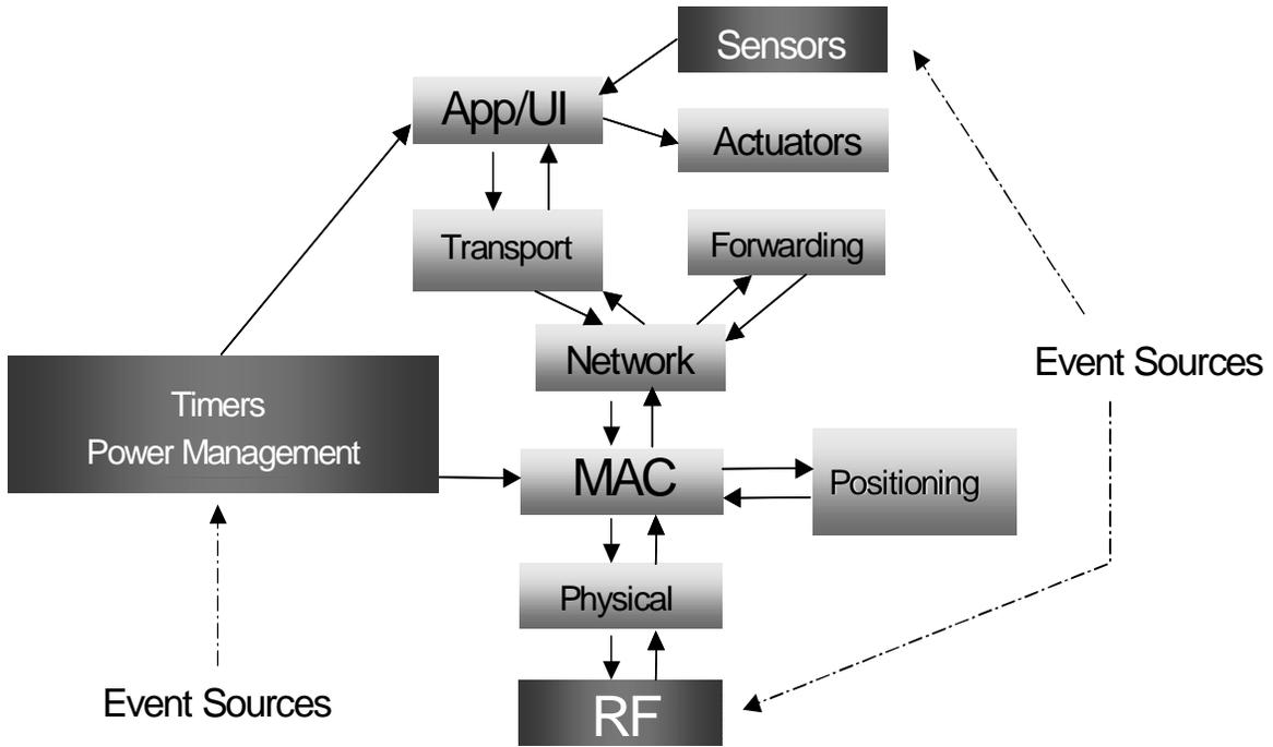
Figure 12.3.5. Block diagram of sensor node.
