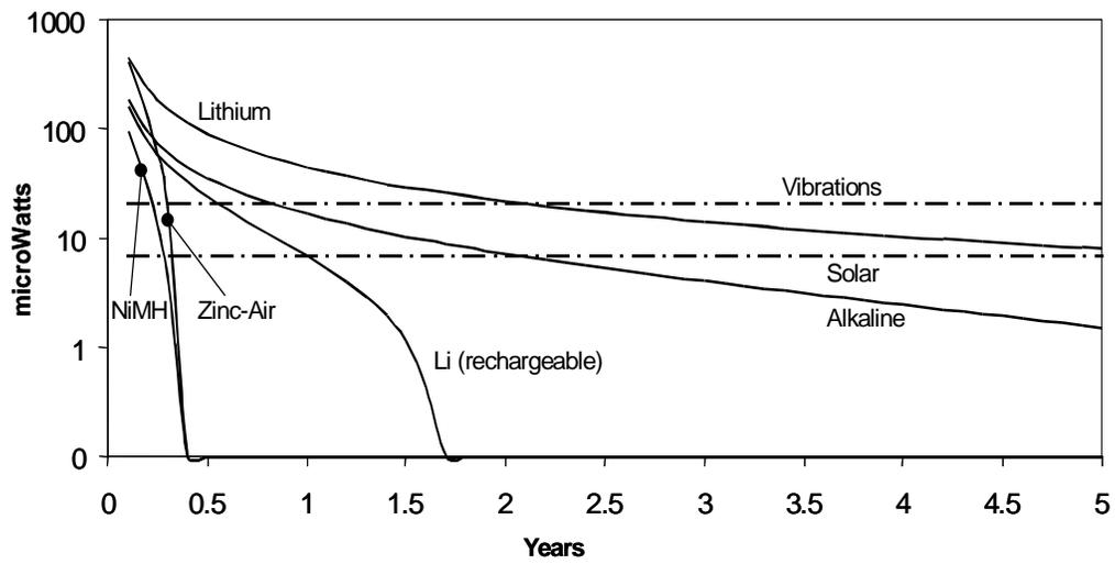
Figure 12.3.1. Battery lifetime ( $0.5 \text{ cm}^3$ ), compared to continuous power sources ( $1 \text{ cm}^2$  solar cell,  $1 \text{ cm}^2$  vibration converter).
