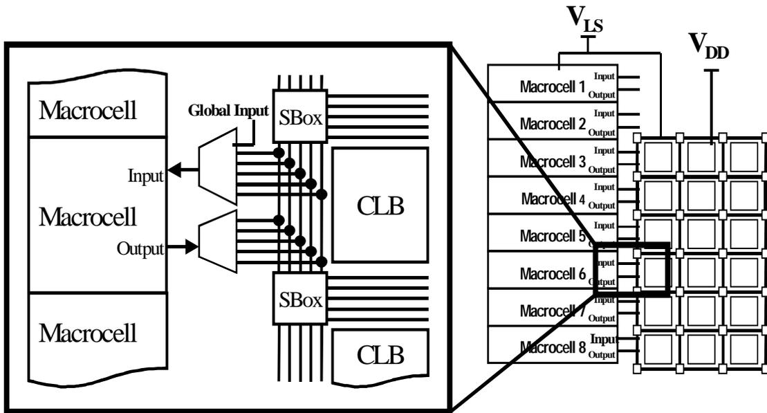
Figure 12.3.4. Hybrid programmable logic array for flexible low-energy implementation of protocol stack.
