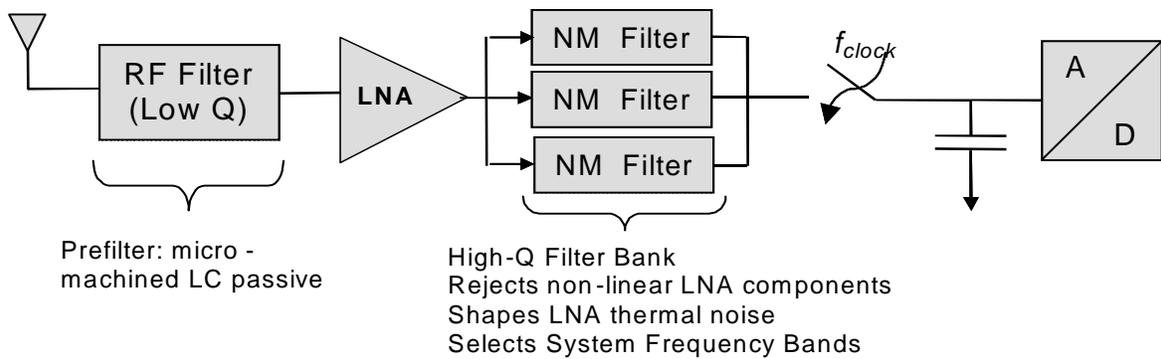
Figure 12.3.2. Sub-sampling RF front-end employing high-Q resonators.
