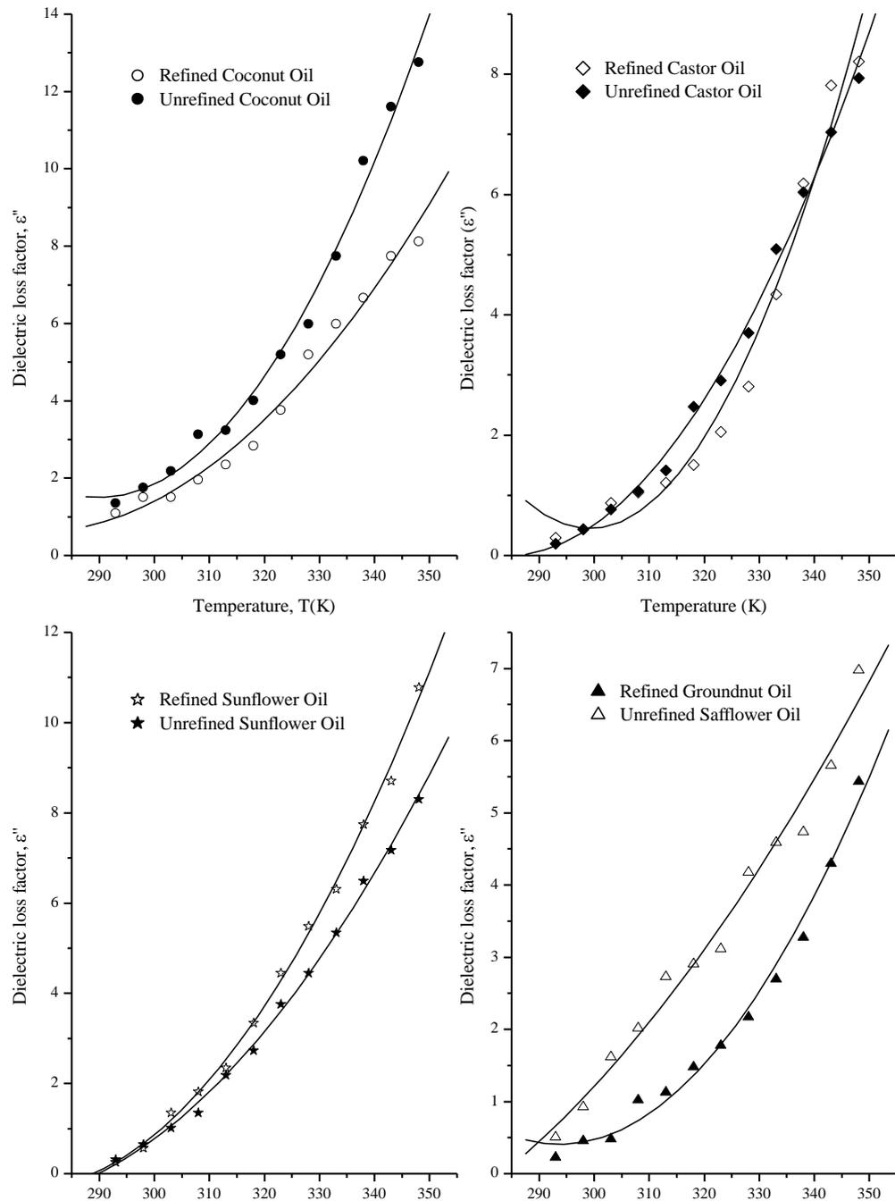
**Fig 2.** Dielectric loss factor as a function of temperature
