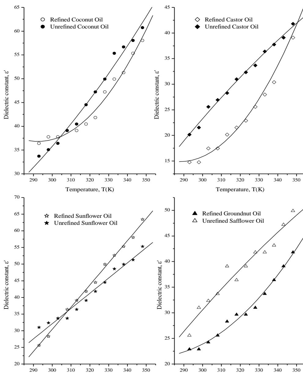
Fig 1. Dielectric constant as a function of temperature
