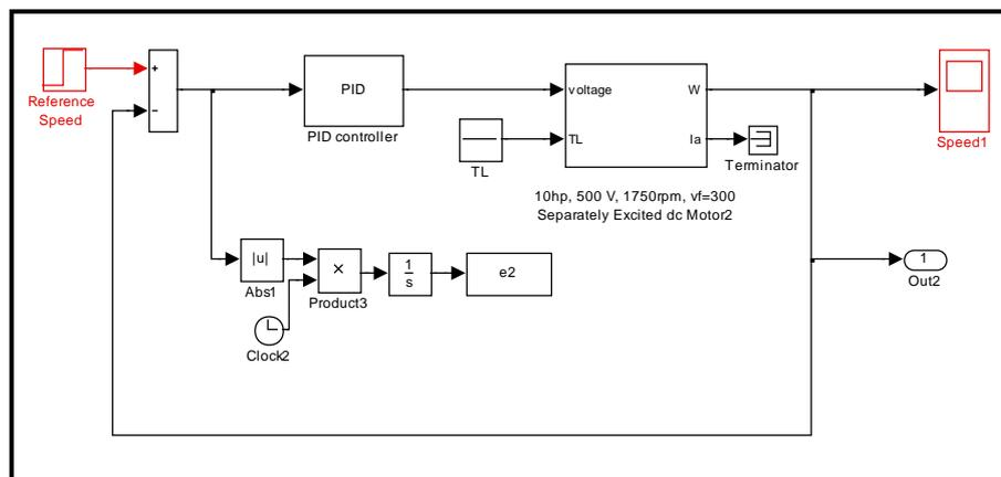
Figure 3: Closed loop speed control system of SEDM
