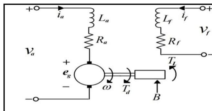
Figure 1: Equivalent circuit of separately excited DC motor
